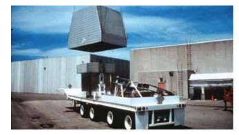
Figure 3: Package and trailer for road transport of used nuclear fuel: OPG (above); Areva (right).
