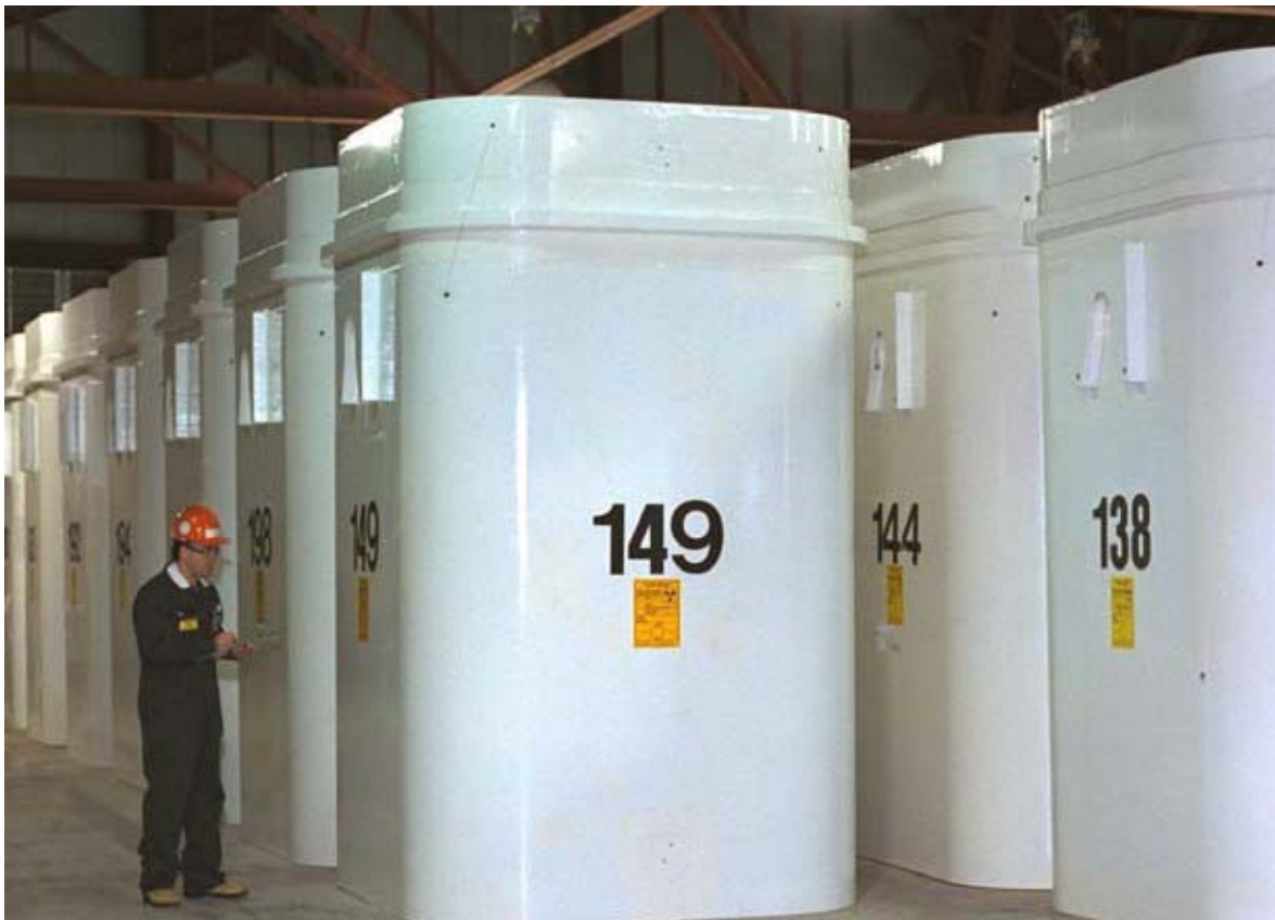
Figure D-6. Dry storage containers holding spent fuel inside the Phase I Building at Pickering NGS (OPG).
