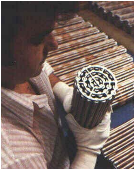
Figure 3. A typical CANDU fuel bundle.
