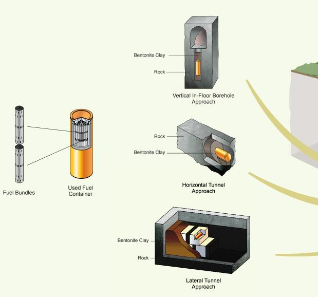
The containers will be placed in vertical boreholes drilled in the floor along the axis of a placement room (in-floor borehole method), or placed horizontally within the confines of a placement room (horizontal tunnel method or lateral tunnel method), depending on the nature of the rock and characteristics of the site.
