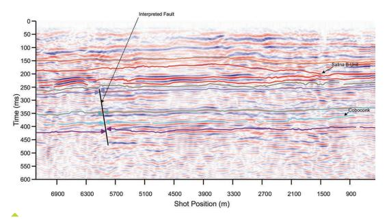
Data from a seismic survey that generates images that show boundaries of rock layers.
