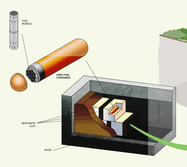
The containers will be placed into a bentonite buffer box in the used fuel packaging plant. These buffer boxes are stacked (two high) in the horizontal placement room, and any spaces are backfilled with bentonite pellets.
