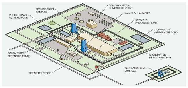
Example of a Layout of APM Surface Facilities for a Deep Geological Repository
