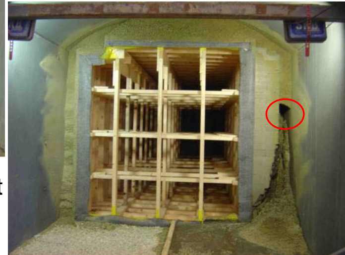
Inflow 2.5 l/min right side Test duration 65 h Initial outflow @ 0.5 h
