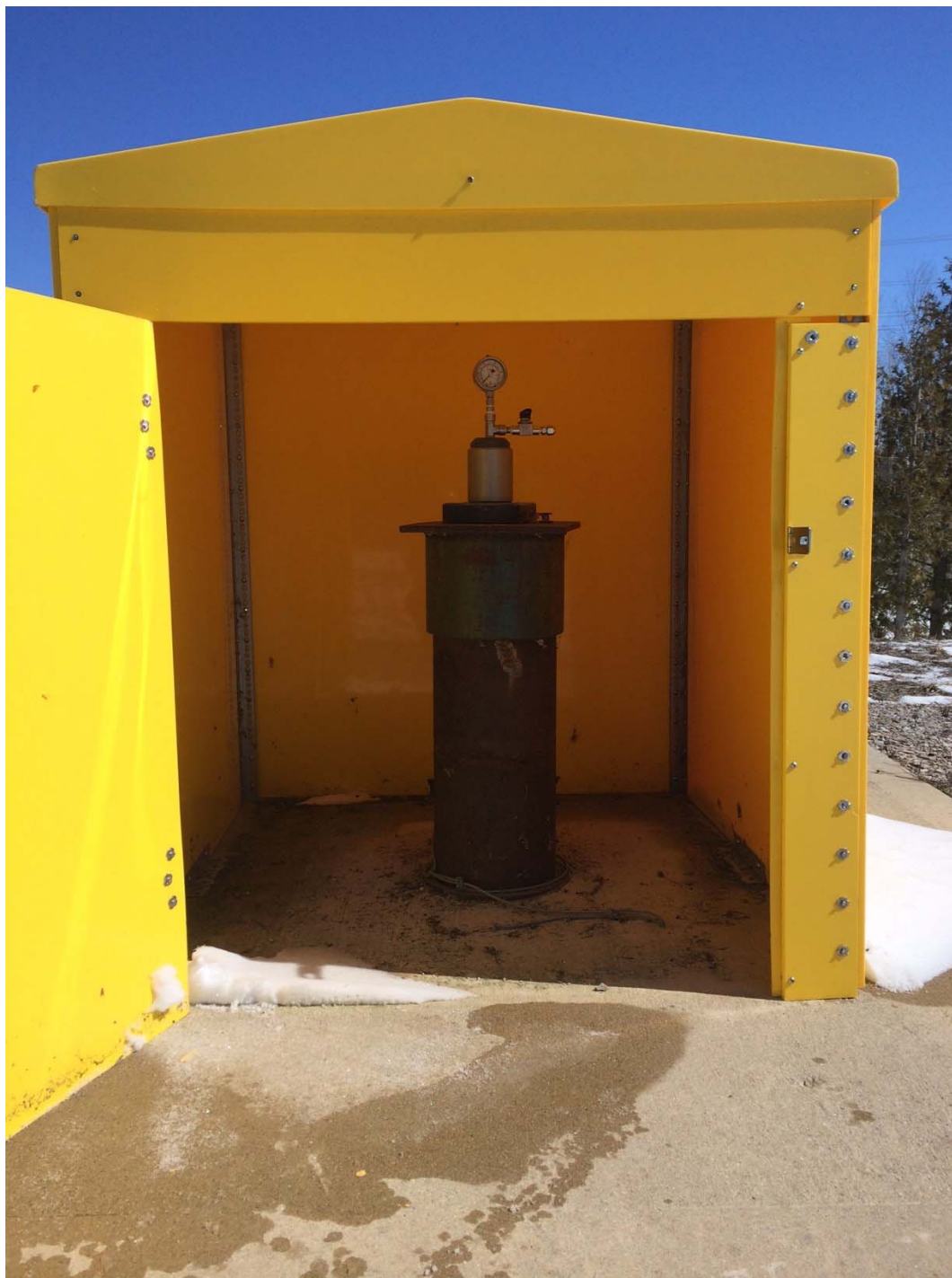
Figure 2: Example of an Enclosure Placed Atop of an Instrumented Well Head
