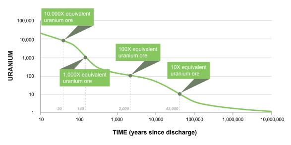
Although its radioactivity level decreases rapidly with time, residual radioactivity (together with some chemical toxicity) persists, and the used fuel remains a potential health risk for many hundreds of thousands of years.
