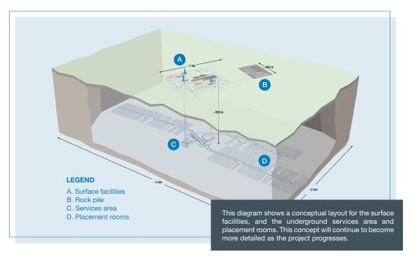
The deep geological repository uses a multiple-barrier system designed to safely contain and isolate used nuclear fuel over the long term. It will be constructed at a depth of approximately 500 metres, depending upon the geology of the site, and consists of a network of placement rooms for the used nuclear fuel. This approach aligns with international best practices.
