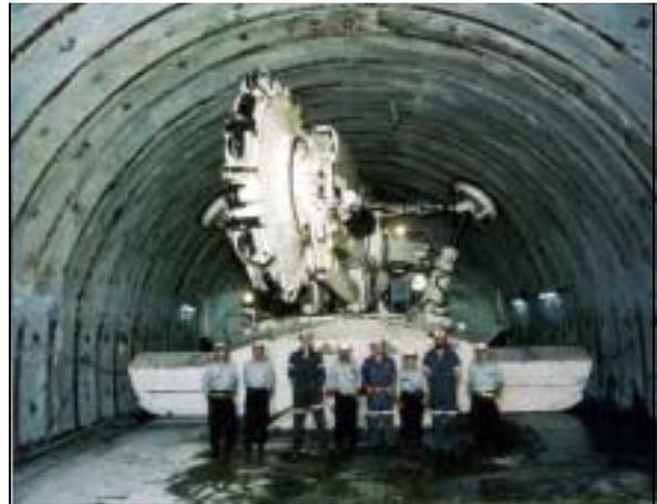
Commercial Mobile Miner, capable of tight radius turns and mining non-circular shapes
