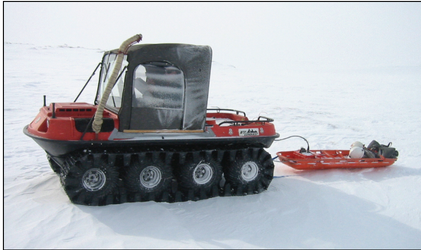
Figure 3: It was possible to conduct the survey under the arctic conditions using a vehicle provided by Kinross Ltd. The main unit of the radar and the batteries were in the warm cabin while the antenna was positioned in the sled. The coordinates and the orientation for the survey lines were obtained from GPS.
