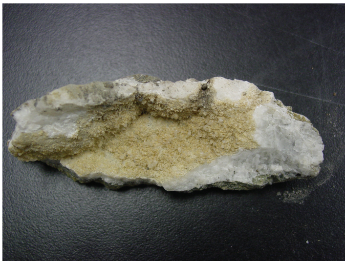
Figure 49: Examples of two calcites found at the Lupin Mine, along the access ramp. (A) Calcite with graphite interfingerings from the 270 m level. (B) Vuggy calcites with a light brown coating (oxy-iron-hydroxides) were found in the upper portions of the mine, like this one from the 440 m level.
