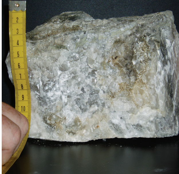
Figure 46: Sample from the large calcite vein found along the ramp at the 540 level in the Lupin Mine.
