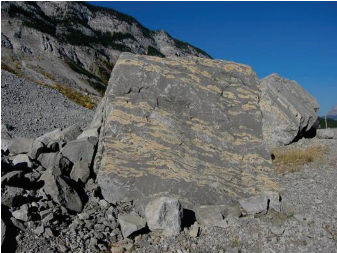
Figure 26: Example of Layering in Dolomitic Limestone Resulting in Anisotropic Properties (R. Read)
