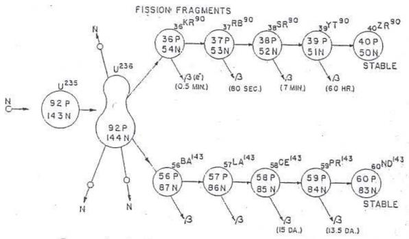
Representing the fission of uranium 235 plus neutron, forming two short radioactive "chains".
