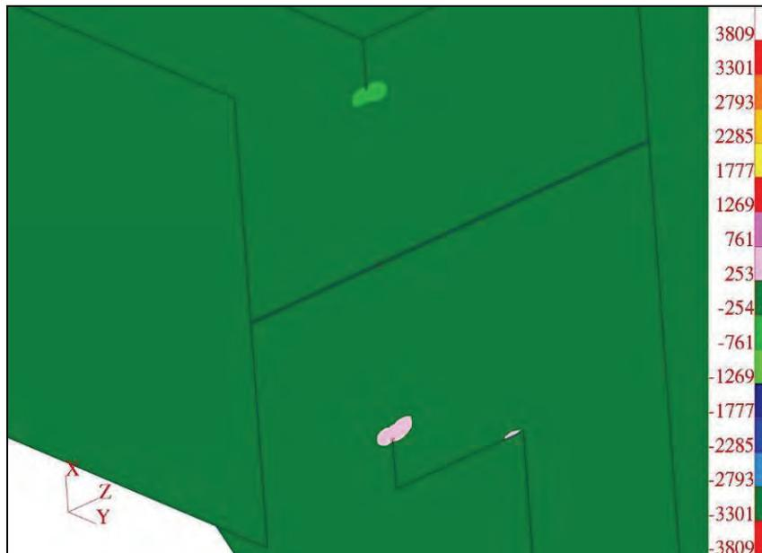
Figure Ac-8: Opening/Closing Stress Component (MPa) (Model II-b)
