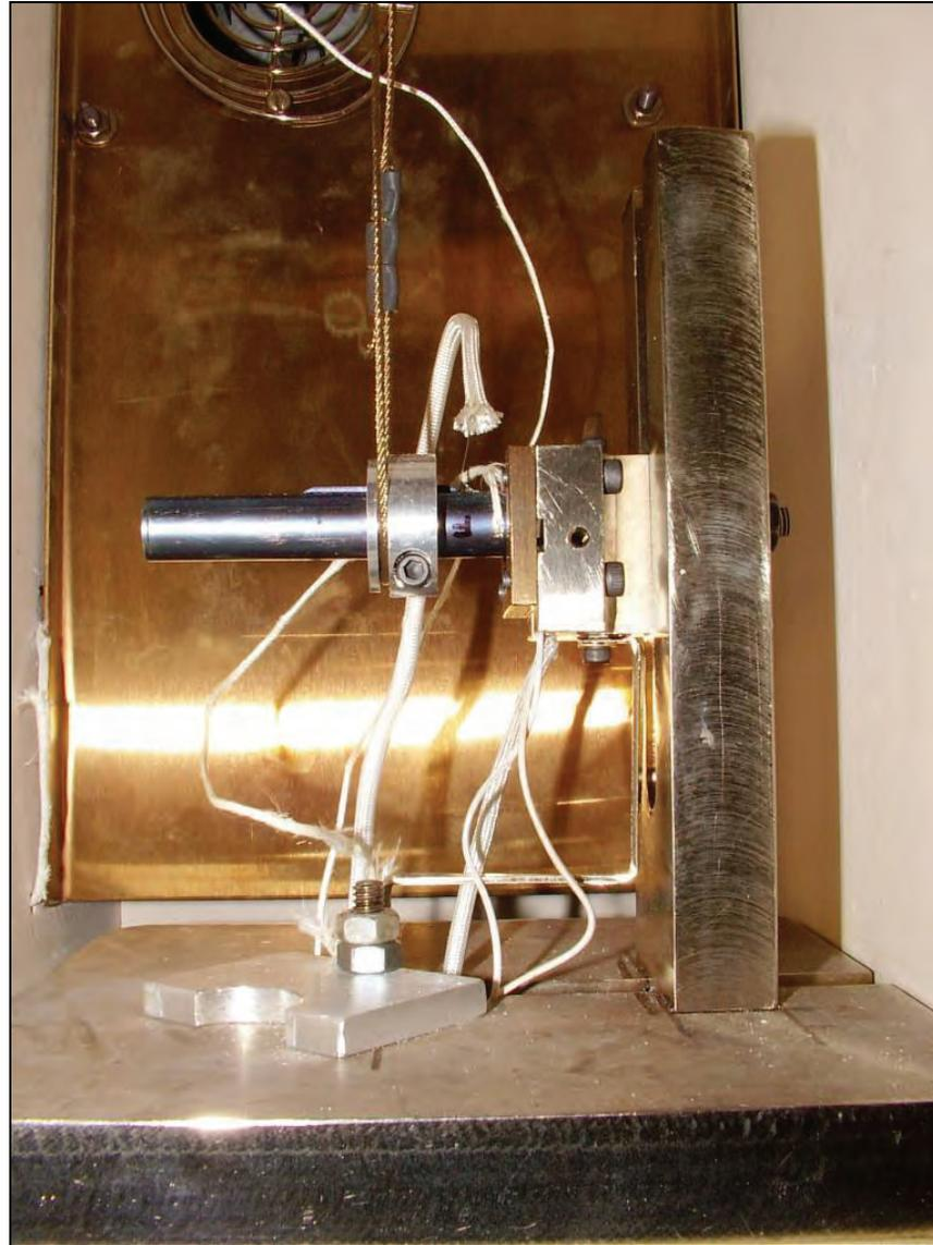
**Figure 9: Photograph Showing the Sample in the Loading Rig under Load**
