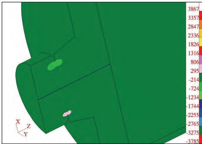
Figure Ac-14: Opening/Closing Stress Component (MPa) (Model IV-a)
