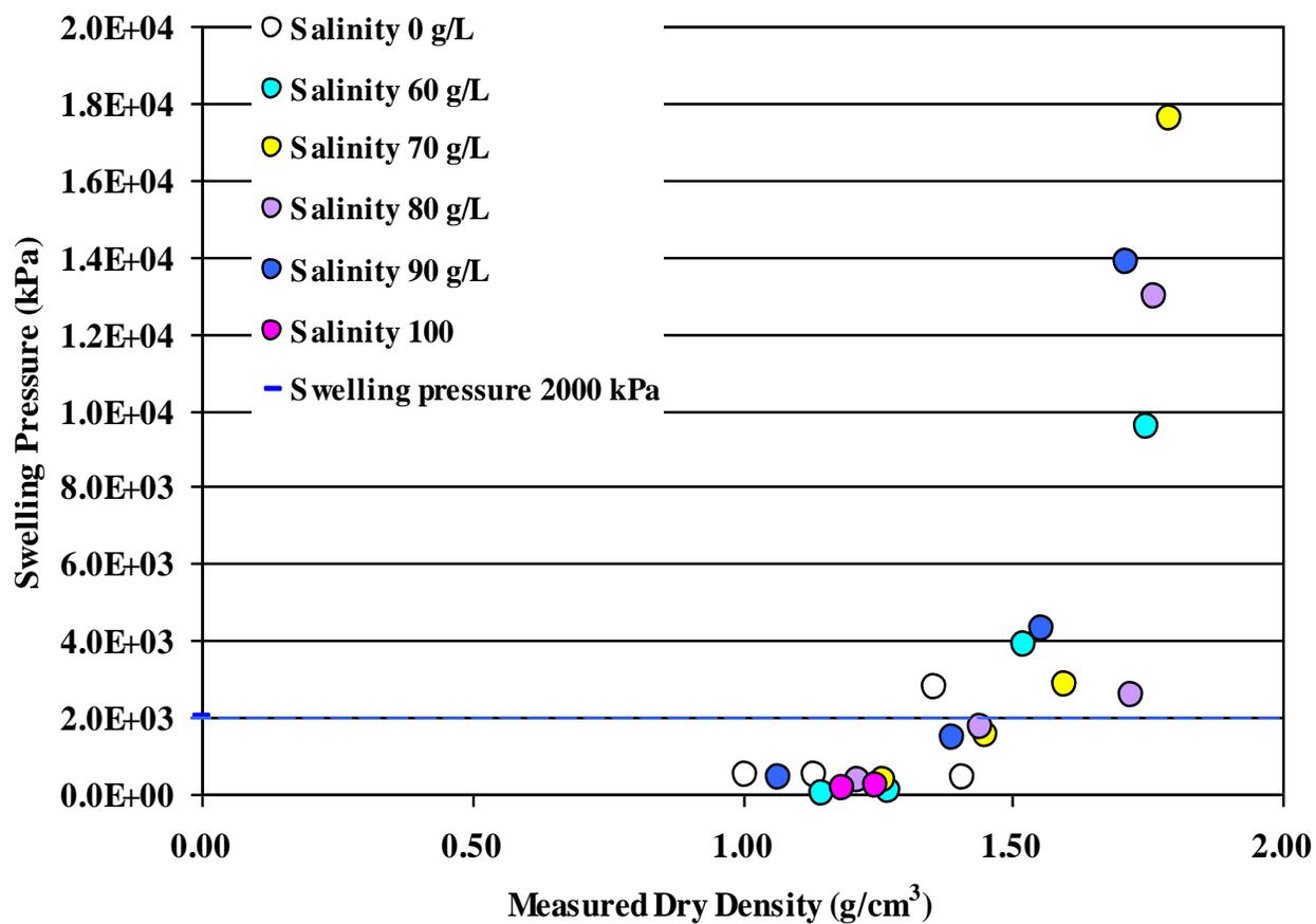
Figure 29: Swelling pressure in compacted bentonite as a function of measured dry density and salinity (new data).
