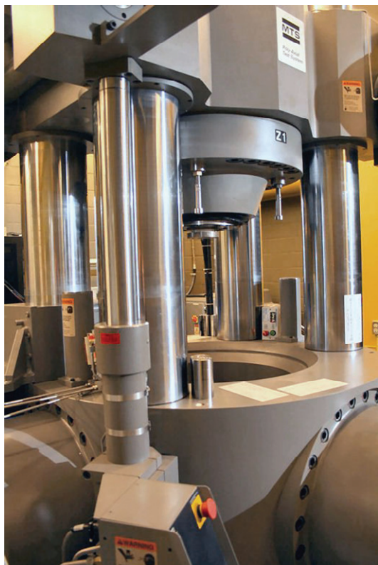
Figure 4.8: THM experimental equipment at the Rock Fracture Dynamics Facility, University of Toronto. (a) Custom-made polyaxial loading machine (MTS Systems Corporation). (b) Polyaxial geophysical imaging cell which provides real-time geophysical monitoring during coupled THM experiments.
