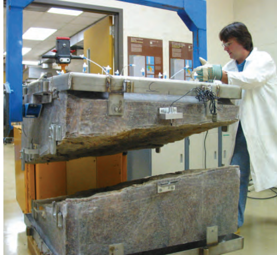
Figure 1: Quarried Block Sample Opened for Inspection of Fracture Surfaces
