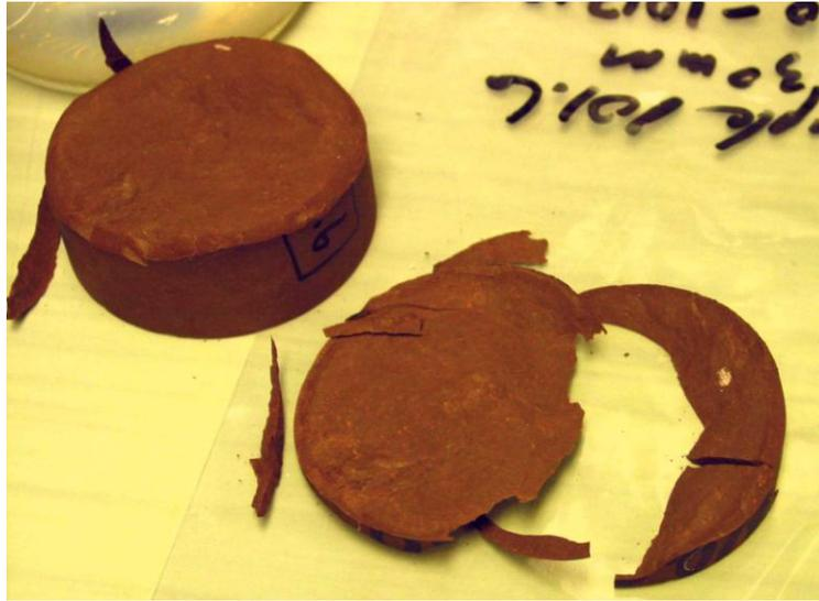
**Figure 3: Examples of Queenston Shale Core Slices Showing Disintegration after Wetting**
