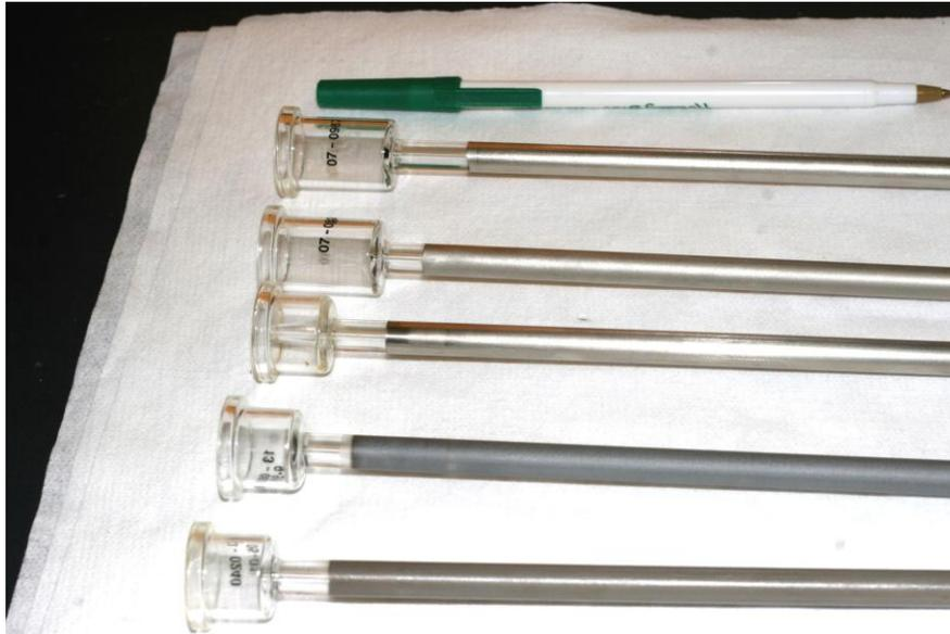
**Figure 9: Penetrometer Stems Used to Hold Samples During MIP Analyses**
