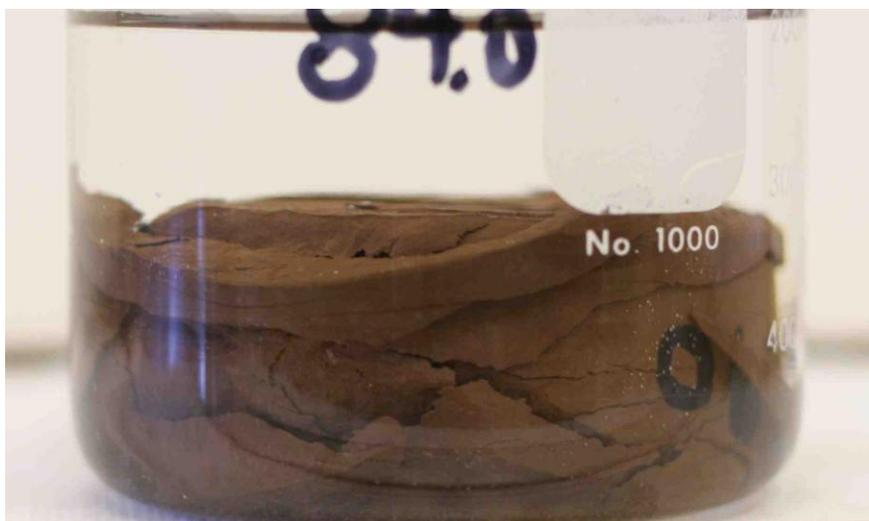
**Figure 23: Core Slice of Queenston Shale Immersed in 170 g/L KNO<sub>3</sub> Showing a Parting Pattern Typical of Unconfined Samples Immersed in Water**
