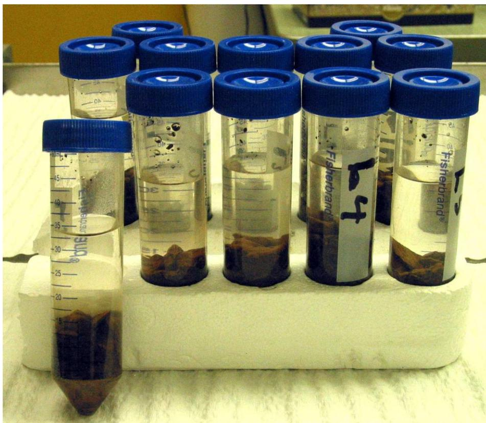
**Figure 19: Shale Samples Being Leached to Determine Pore Fluid Composition**
