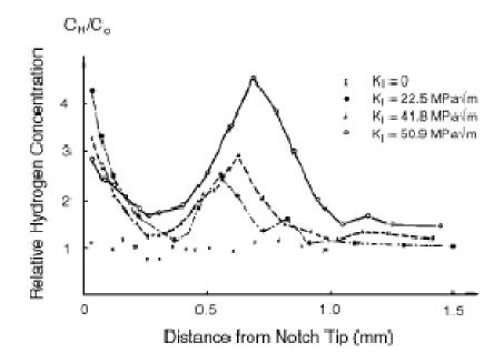
Figure 16: Measured Accumulation of Hydrogen Ahead of a Notch in Carbon Steel as a Function of Stress Intensity Factor (Yu et al. 1997).
