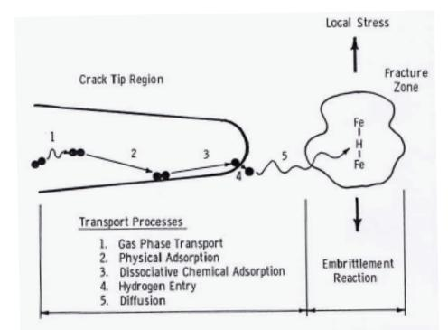
Figure 4: Processes Involved in the Absorption of Hydrogen from the Gas Phase and the Subsequent Embrittlement Reaction (Wei and Gao 1985).
