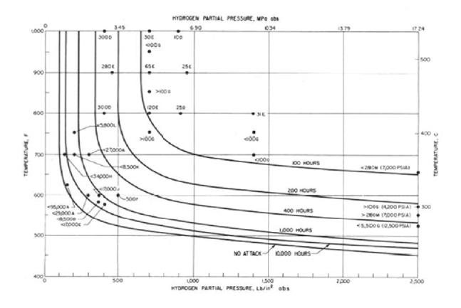
Figure 19: Nelson Curves for Carbon Steel as a Function of Exposure Time. The maximum  $H_2$  pressure in the repository of 8 MPa is equivalent to a pressure of 1160 lb/in<sup>2</sup> (Nelson 1977).
