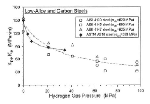
Figure 24: Dependence of the Threshold Stress Intensity Factor for Crack Growth  $(K_{IH})$  for ASTM A516 Carbon Steel and for Crack Arrest  $(K_{TH})$  for Three Low-alloy Steels on Hydrogen Pressure (Gangloff 2009).
