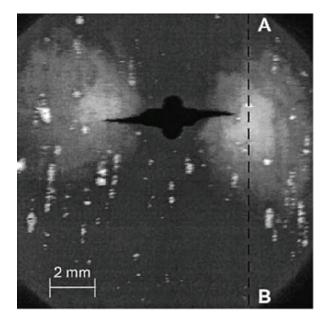
Figure 15: Photoelectrochemical Image of Hydrogen Concentrating at the Locations of Highest Stress in the Fracture Process Zone Ahead of the Crack Tip (Razzini et al. 1999).
