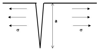
(a) Edge crack of depth a in a semi-infinite plane subject to uniaxial tensile stress  $\sigma.$
