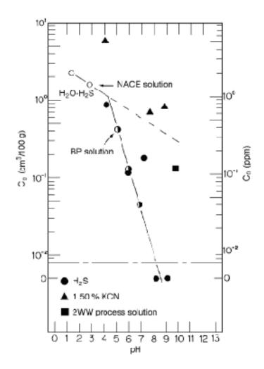
Figure 5: Dependence of the Lattice Hydrogen Concentration on Solution pH in the Presence of 0.01 MPa  $H_2S$  at 25°C (Yamakawa and Nishimura 1999). The BP solution is based on artificial seawater and the NACE solution contains acetic acid and NaCl.
