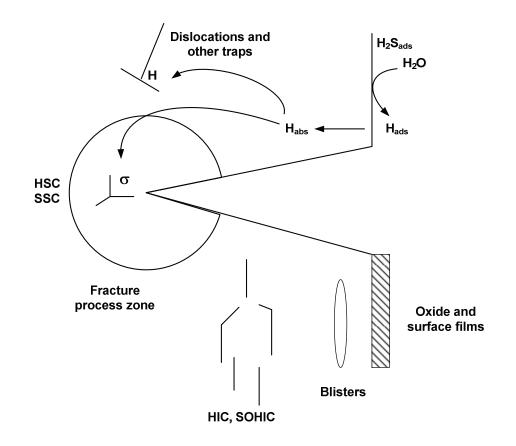
Figure 1: Schematic of the Processes Involved in the Hydrogen Degradation of Steel.
