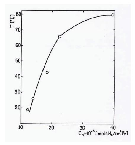
Figure 22: Temperature Dependence of the Critical Hydrogen Concentration ( $C_{\kappa}$ ) for Blister Formation on Armco Iron (Beck et al. 1966). A H concentration of 10<sup>-8</sup> mol H<sub>2</sub>·cm<sup>-3</sup> Fe corresponds to 0.0025 µg·g<sup>-1</sup>.
