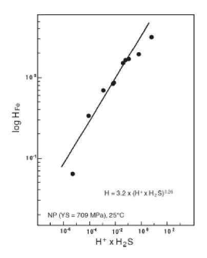
Figure 6: Dependence of the Lattice Hydrogen Concentration on pH and Dissolved Sulphide Concentration at 25°C (Asahi et al. 1994). The hydrogen concentration  $H_{Fe}$  is in units of  $\mu g \cdot g^{-1}$  and the concentrations of  $H^+$  and dissolved  $H_2S$  in mol·dm<sup>-3</sup> and  $\mu g \cdot g^{-1}$ , respectively.
