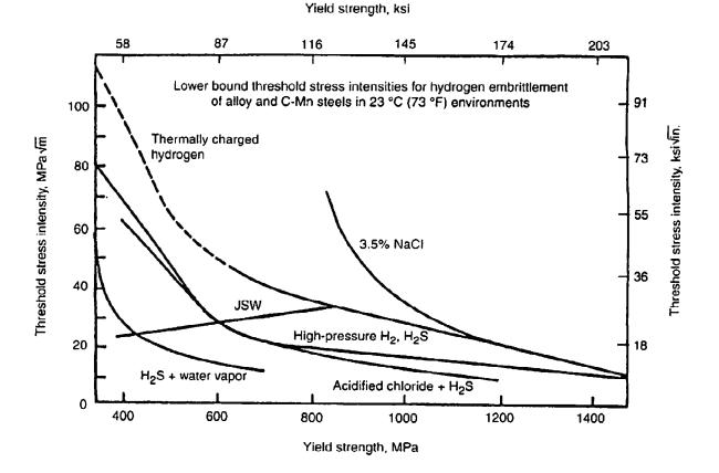
Figure 23: Dependence of the Threshold Stress Intensity Factor for Hydrogen Embrittlement of Alloy and C-Mn Steels at 23°C (Gangloff 2009).
