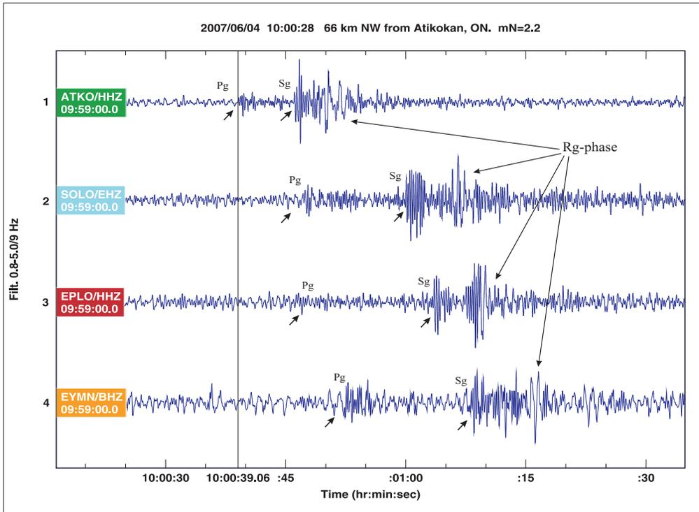
Figure 8: Rg Surface Waves from the  $m_N$  2.2 on 2007/06/04 NW of Atikokan, ON
