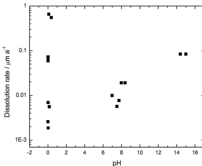
**Figure 26: Dissolution (passive corrosion) rates of anodically grown oxides on Zr as a function of pH (Mogoda 1999a, El-Mahdy and Mahmoud 1998, El-Mahdy et al. 1996, Huot 1992, Allah et al. 1989)**
