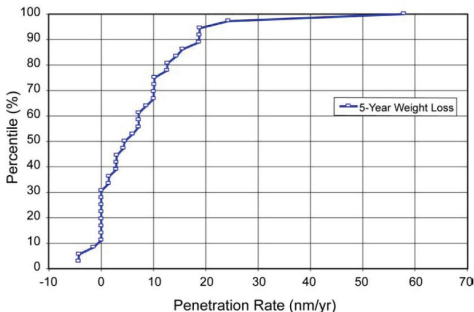
**Figure 25: Distribution of the passive corrosion rates of the Pd-containing Ti alloy, Grade-16, measured after exposure to a number of concentrated saline groundwaters (Hua et al. 2005 a, b, c)**
