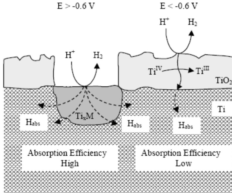
Figure 11: Schematic illustrating the low efficiency of H absorption under passive conditions on Ti and the possibility of a higher absorption efficiency through the locations of cathodically-activated secondary phase precipitates (SPPs)
