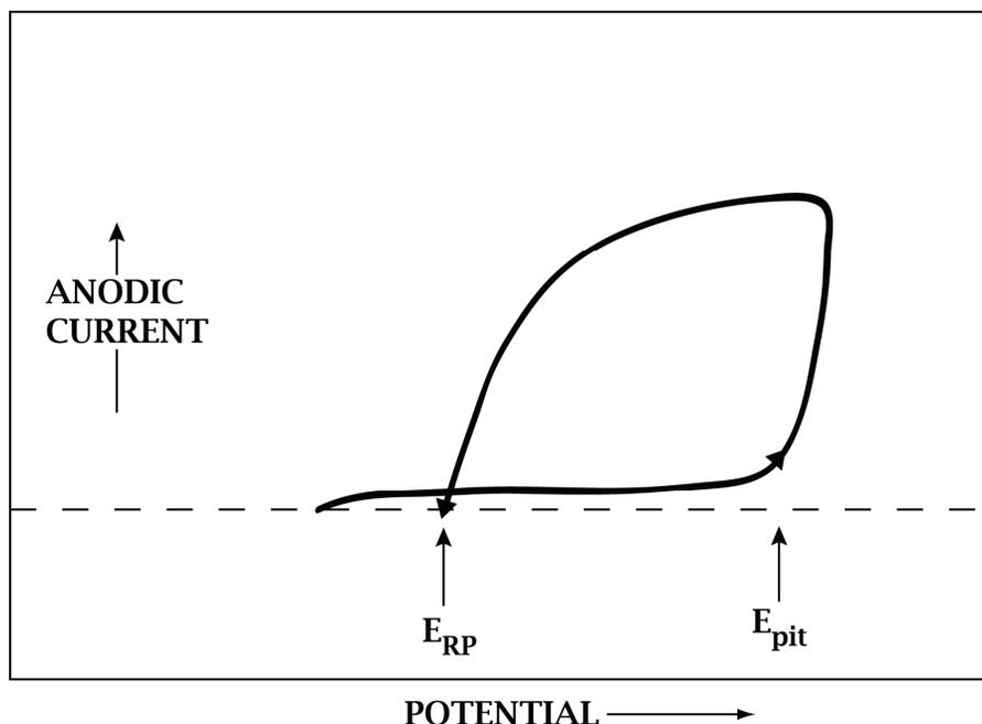
**Figure 19: Illustration showing the form of the current-potential relationship observed in a potentiodynamic scan recorded to determine the pitting breakdown potential ( $E_{pit}$ ) and the repassivation potential ( $E_{RP}$ )**
