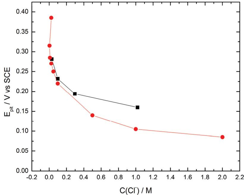
**Figure 20: Pitting breakdown potentials recorded as a function chloride concentration (C); ○-Knittel and Bronson (1984); □ Jangg et al. (1978)**
