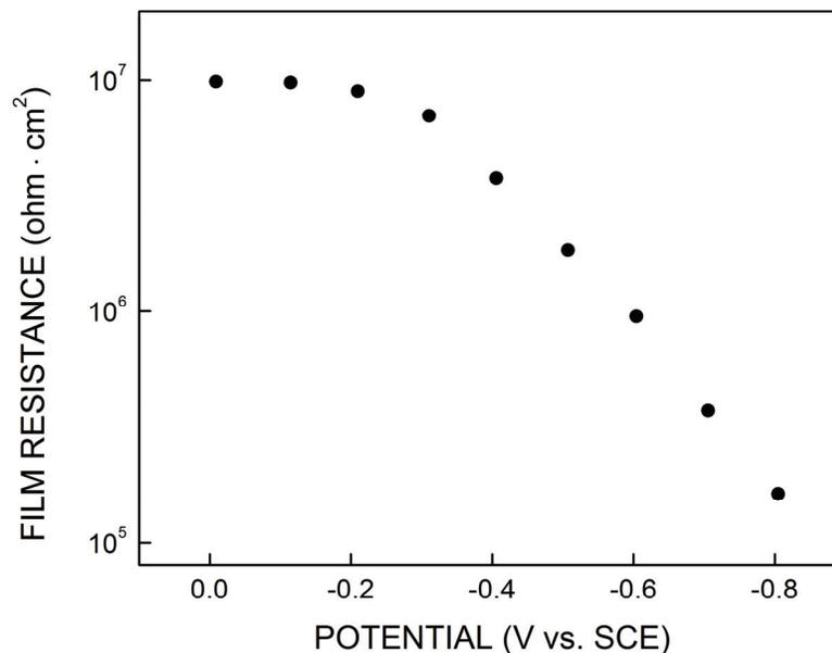
**Figure 6: Variation of the oxide film resistance on Grade-2 Ti as a function of applied potential in a deaerated neutral 0.27 mol/L NaCl solution. The resistance was determined by electrochemical impedance spectroscopy on an oxide pre-grown by anodic oxidation at 0.6V (vs SCE) for 48 hours (Zeng 2009)**
