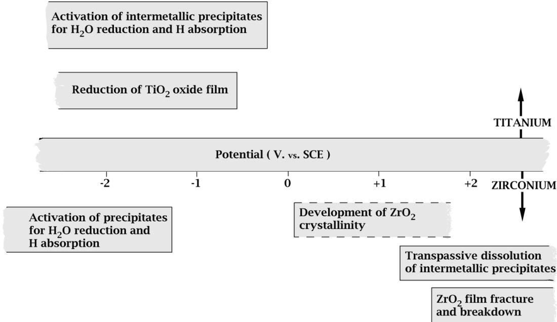
**Figure 13: Schematic showing the potential ranges within which various processes can occur on anodically or cathodically polarized Ti and Zr alloys**
