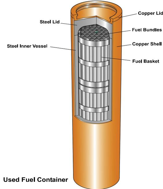
**Figure 15: Cut away view of the used fuel container showing the inner and outer vessels and the fuel bundles (Shoesmith 2007)**
