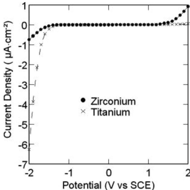
**Figure 1: Polarization behaviour of Ti and Zr in neutral 0.1 mol/L KClO<sub>4</sub> solution (Noël et al. 2008)**
