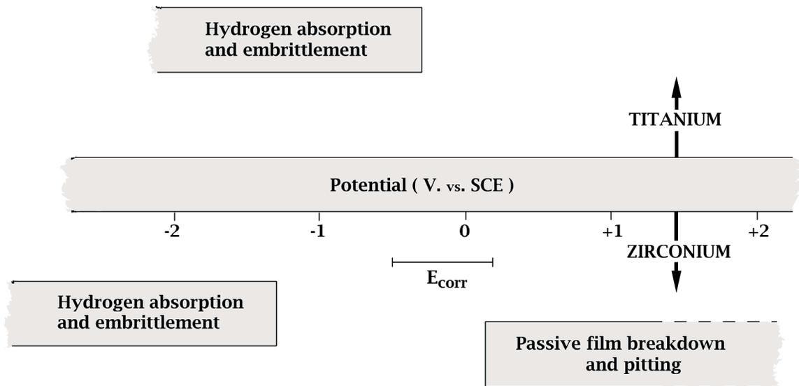
**Figure 18: Schematic showing the potential ranges within which passive film breakdown/pitting and H absorption/embrittlement could occur on Ti and Zr alloys. The bar marked  $E_{CORR}$ , shows the range of corrosion potentials measured on Zr alloys in neutral solution**
