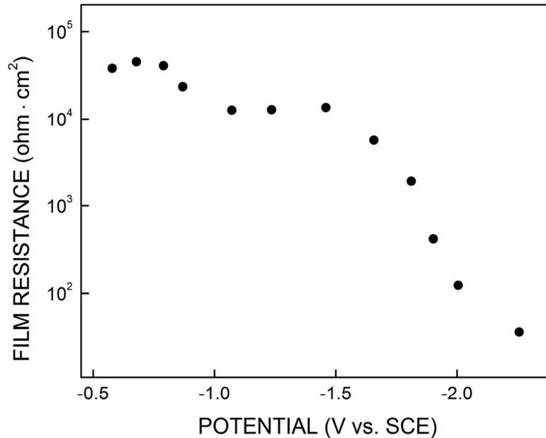
**Figure 7: Variation of the oxide film resistance on Zr-2 as a function of applied potential in a deaerated neutral 0.1 mol/L Na<sub>2</sub>SO<sub>4</sub> solution. The resistance was determined by electrochemical impedance spectroscopy on an oxide pre-grown in air for 24 hours prior to exposure to the solution (Nowierski et al. 2009a, b)**
