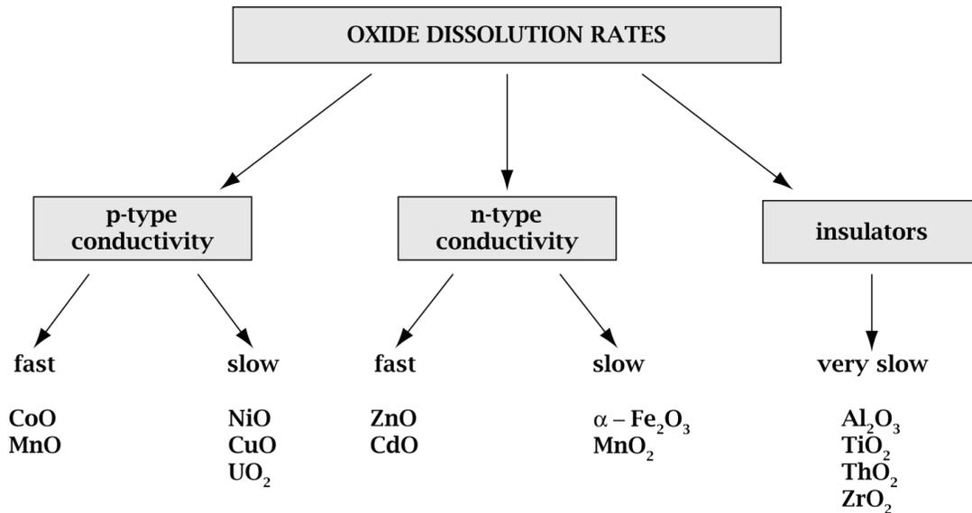
**Figure 24: Categorization of the dissolution rates of various oxides separated according to their conductivity type (Segall et al. 1988)**
