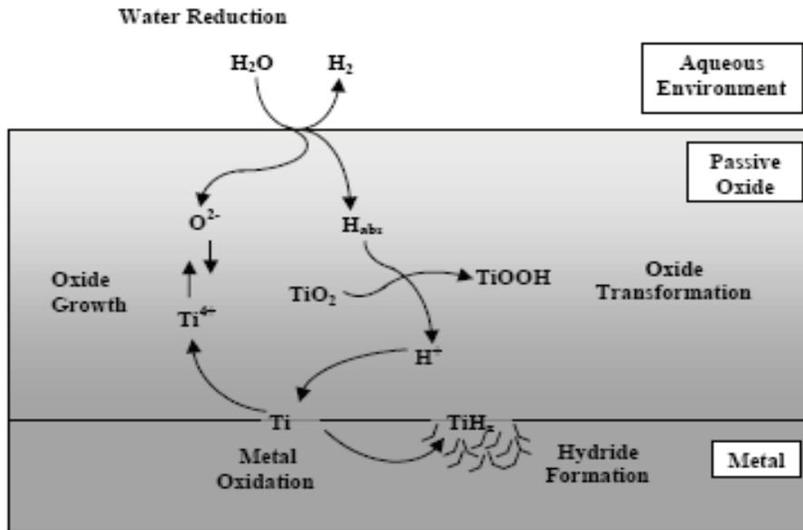
**Figure 8: Schematic illustration of the transformations in a  $\text{TiO}_2$  film on Ti occurring under cathodic polarization leading to the absorption of H into the metal and the formation of hydrides**
