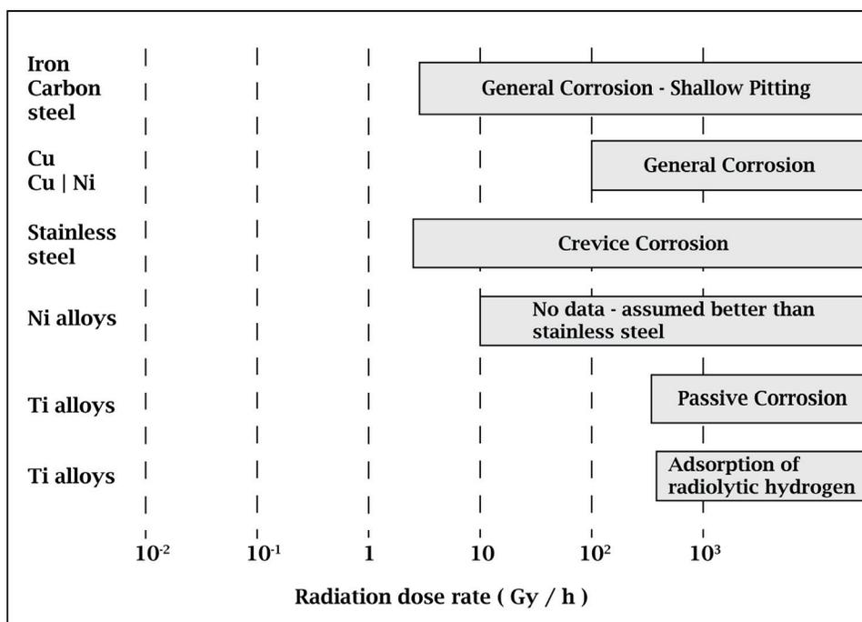
**Figure 21: Summary showing the gamma radiation dose rate ranges (shaded areas) within which a measurable influence of radiation on various corrosion processes on various materials has been observed (Shoesmith and King 1999). At dose rates below these regions experiments have revealed no observable radiation effect.**
