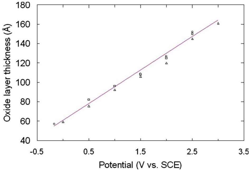
**Figure 4: Oxide layer thickness, determined in neutron reflectometry experiments, as a function of applied potential on Zr in a neutral 0.1 mol/L Na<sub>2</sub>SO<sub>4</sub> solution. The symbols,  $\Delta$   $\square$   $\circ$  show that, while a slight thickening of the oxide occurs with time (6, ~12, ~18 hours, respectively) the thickness has almost achieved a steady-state value (Noël et al. 2008)**
