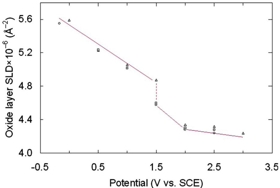
**Figure 5: The scattering length density (SLD) of the oxide film on Zr determined by neutron reflectometry after anodic oxidation at various applied potentials. The data points have the same significance as in Figure 4. The decrease in SLD shows that the hydrogen content of the oxide increases steadily as the potential increases up to ~1.5V, and then suddenly increases as the film undergoes fracture (Noël et al. 2008)**
