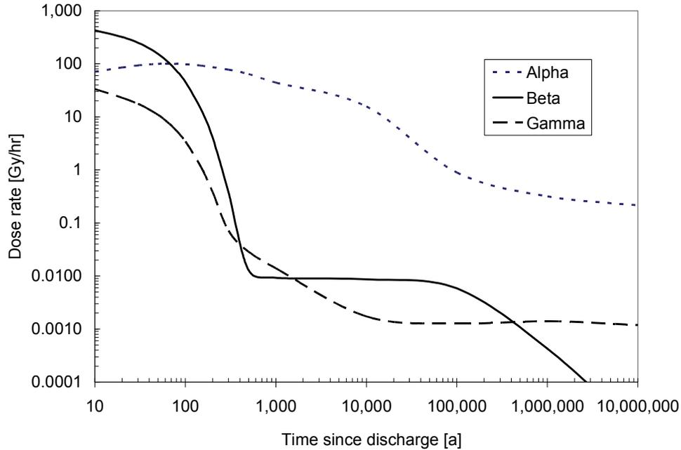
**Figure 17: Alpha, beta and gamma radiation dose rates calculated as a function of time for a layer of water in contact with a CANDU fuel bundle with a burnup of 220 MWh/kgU (Shoemith 2008)**
