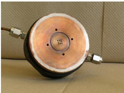
**Figure 6 a: Upper compartment of the copper cell without the palladium membrane**
