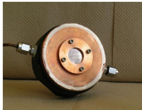
**Figure 6 b: Upper compartment of the copper cell with the palladium membrane mounted**
