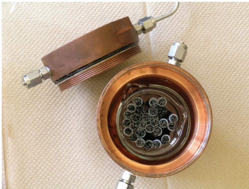
**Figure 5:** Prepared wires in beaker, placed in the copper cell
