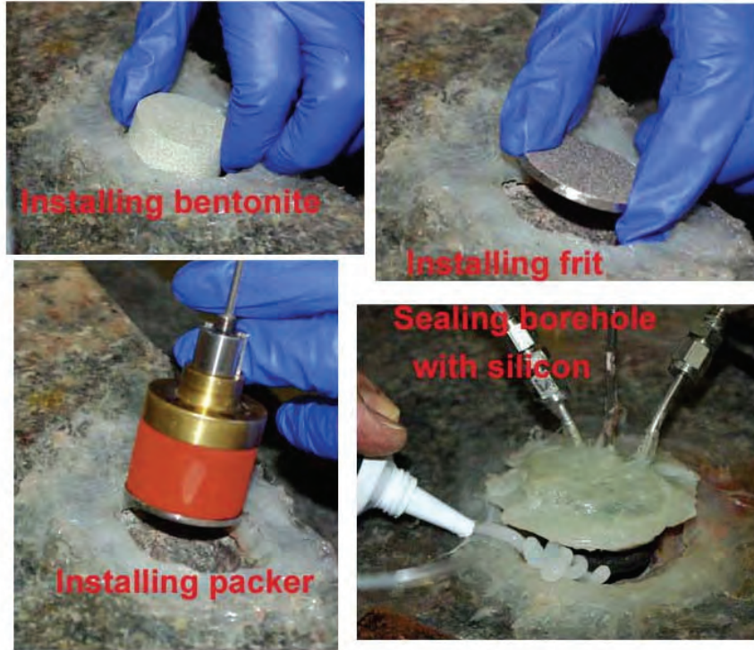
Figure 22: Installation of Bentonite Plugs, Stainless Steel Frits, and Packer Assemblies into L1 and L3 Boreholes.
