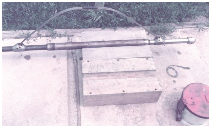
Figure 3.5-6: Gamma Density probe in aluminium calibration block. (Golder Associates)
