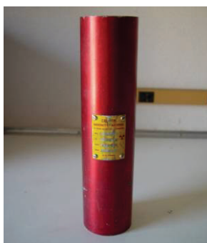
Figure 3.4-5: Photograph of a typical 10 uCi gamma check source. (Golder Associates)
