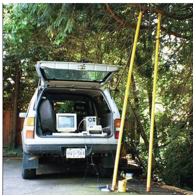
Figure 5.14-5: Normal mode helical electrical antenna system and instrumentation for cross-hole EM. (Groom and Candy, 2001)
