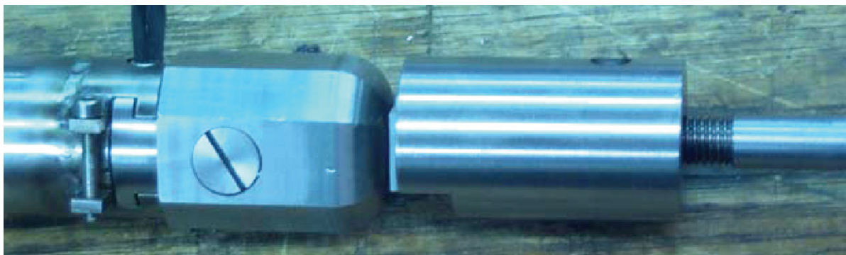
Figure 3.5-5: Photograph showing the end of a compensated density tool with the source holder "bull plug". (Mount Sopris Instrument Co.)
