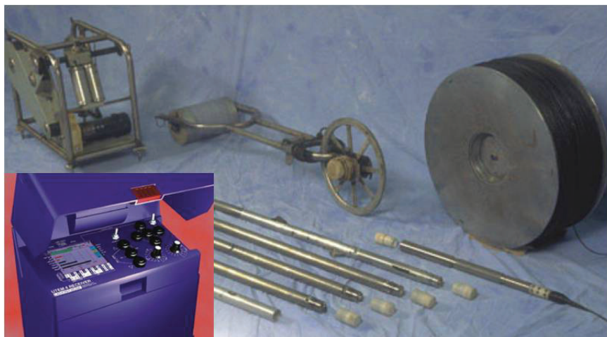
Figure 5.13-1: The BH UTEM4 borehole TDEM receiver system. (Lamontagne Geophysics Ltd.)
