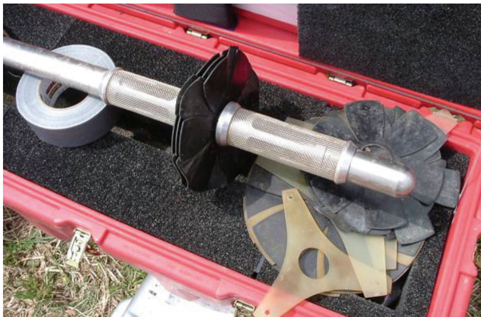
Figure 4.4-1: Mount Sopris heat pulse flow meter model HFP-2293. (USGS)
