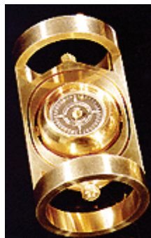
Figure 3.1-2: A Tropari borehole orientation device. (Pajari Instruments Ltd.)
