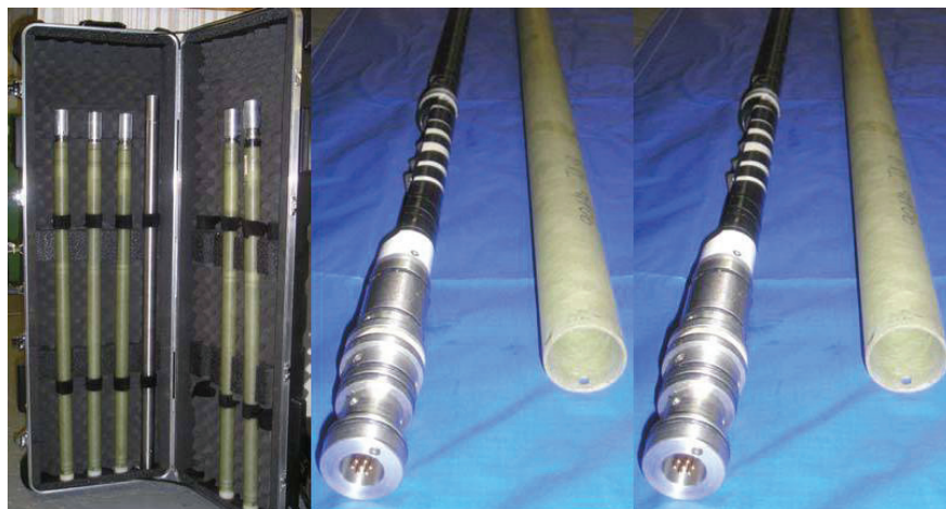
Figure 5.14-4: The Crosswell 3D RIM system antenna assemblies. (Stolar Research Corp.)
