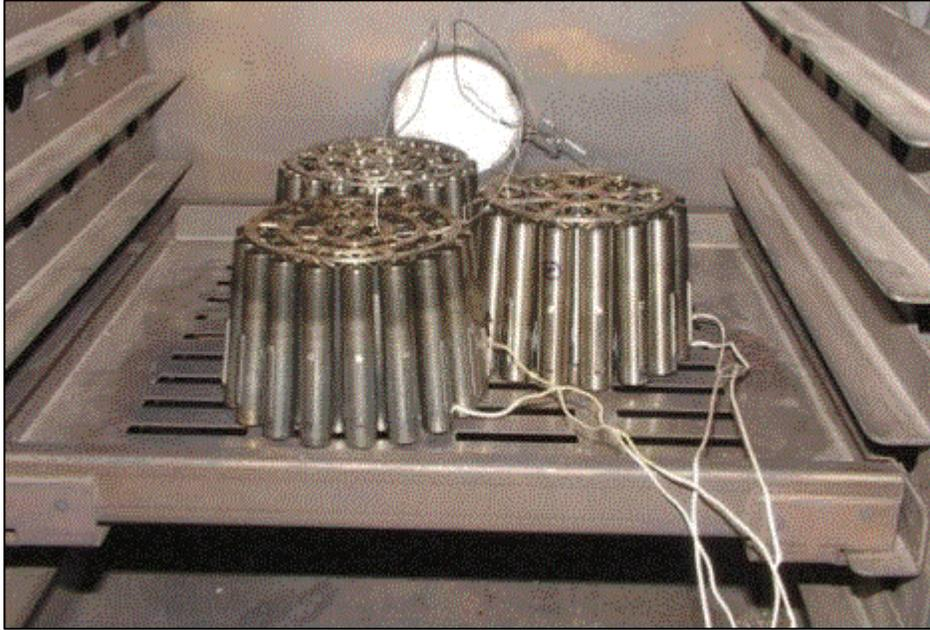
(a) End portion of the fuel bundles with surface hydride layer inside the oven for diffusion anneal
