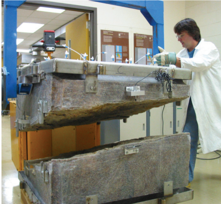
Figure 6.6: Quarried Block sample opened for inspection of fracture surfaces
