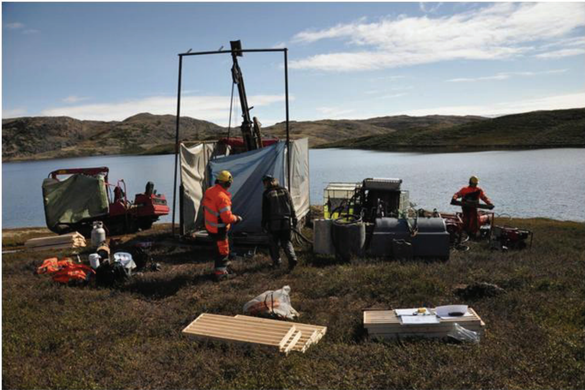
Figure 6.13: Drilling of an inclined borehole near a talik lake west of the ice margin as part of the Greenland Analogue Project 2009 field campaign.
