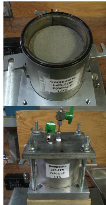
Figure 1: Backfill Clay Block-Bentonite Pellet Assembly in the Modified Cell
