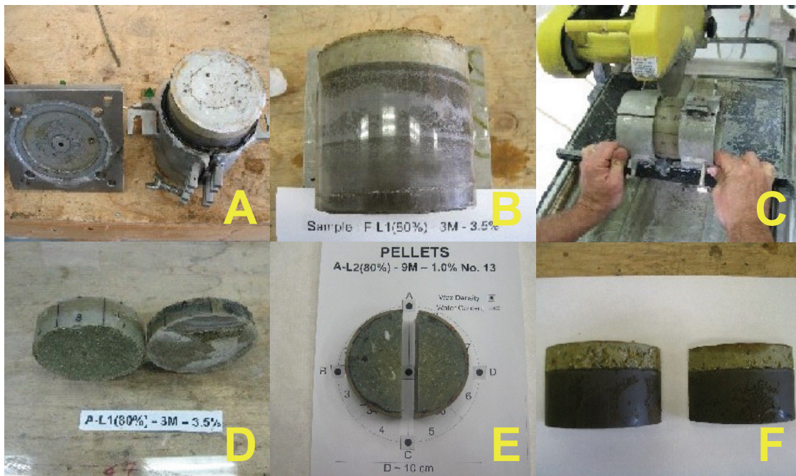
Figure 3: Dismantling of a Testing Cell
