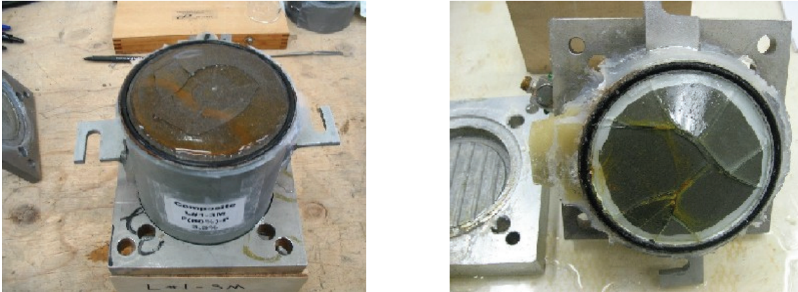
Figure 7: Samples Showing Mechanical Failure at the Top (Left) and Bottom (Right)
