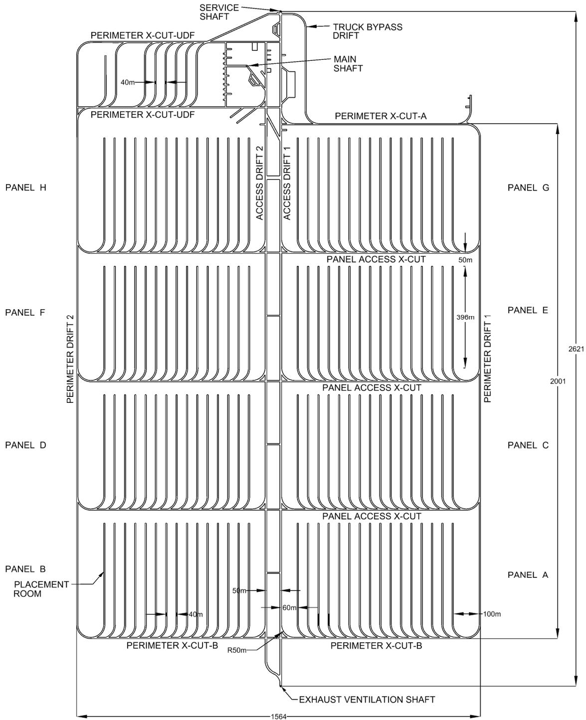
**Figure 2: Underground Repository Layout for the In-floor Borehole Placement Method.**
