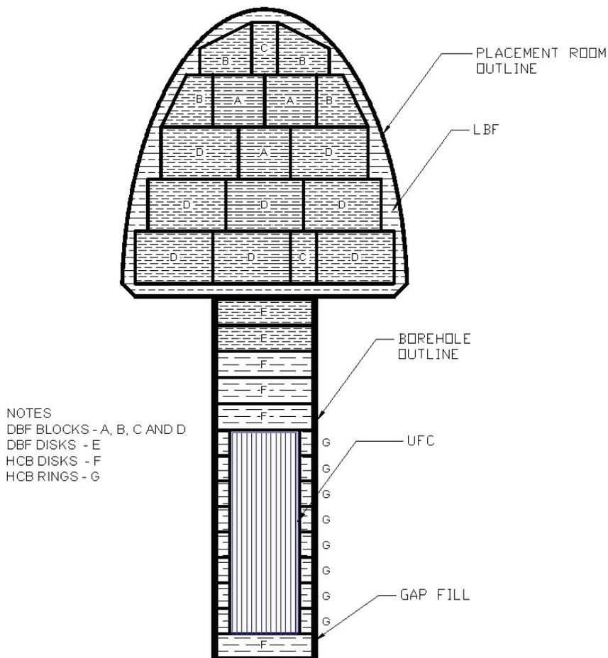
Figure 6: Cross Section of a Filled Placement Room Along the Borehole Axis
