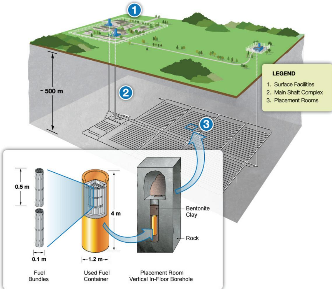
**Figure 1: Conceptual Design for a Deep Geological Repository in Crystalline Rock with In-floor Borehole Placement of Used Fuel Containers.**
