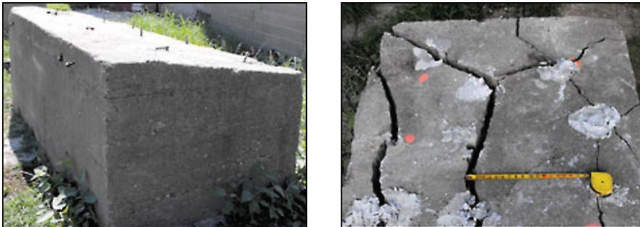
**Figure 5: Use of Expansive Demolition Agent in Concrete**
