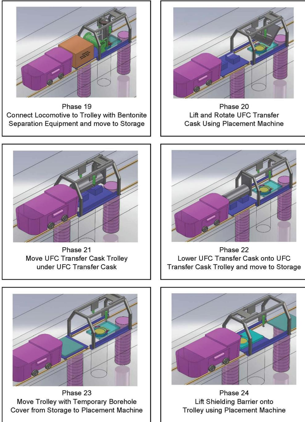
Figure 12: Container Retrieval Sequence of Operations (concluded).
