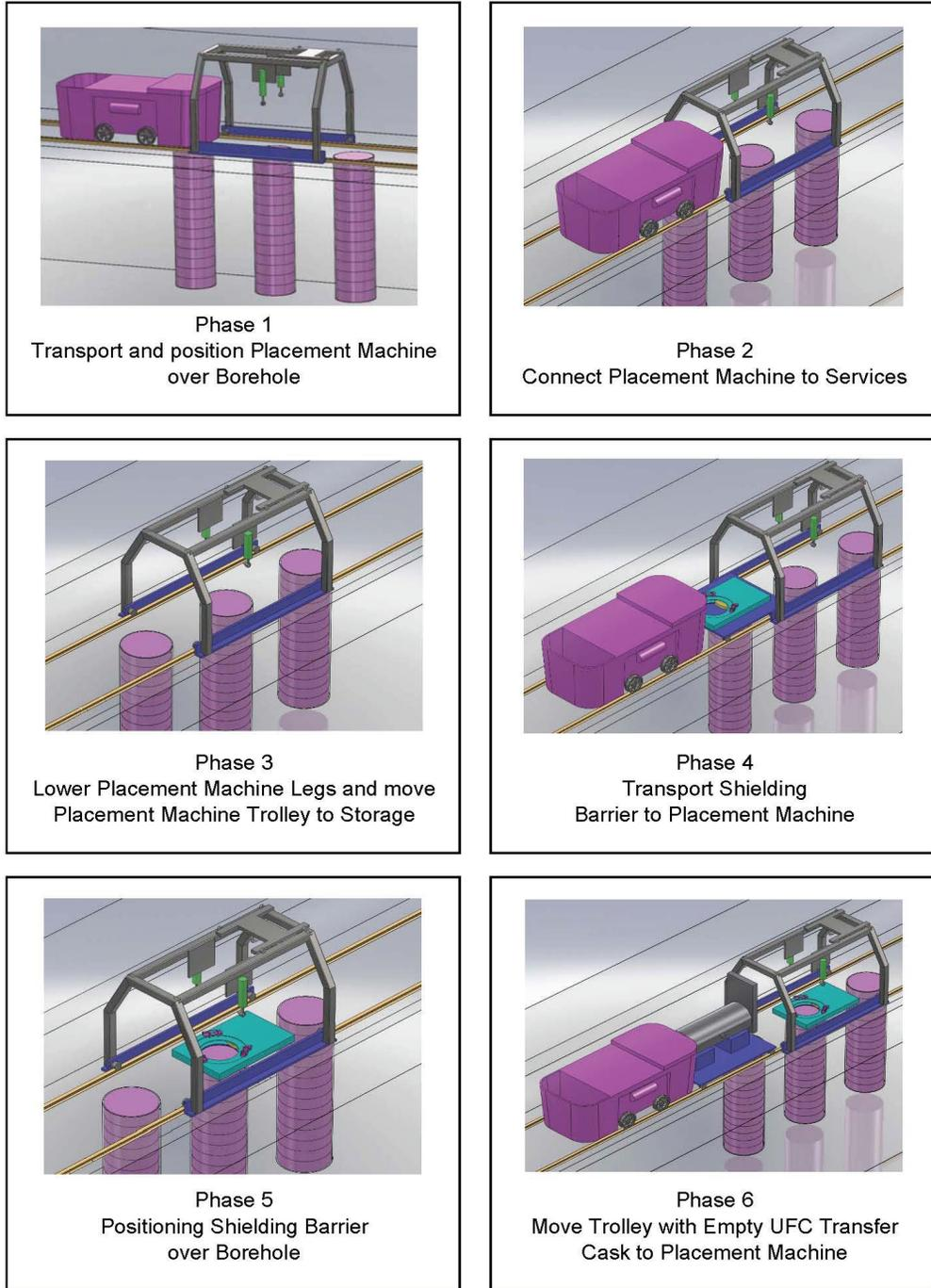
**Figure 12: Container Retrieval Sequence of Operations**
