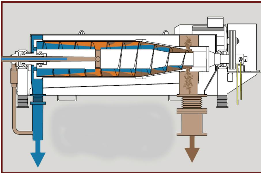
**Figure 9: Diagram of Bentonite Decanting Centrifuge**
