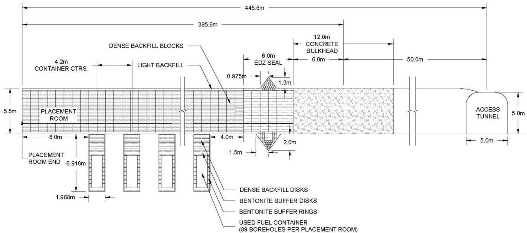
**Figure 3: Repository Placement Room Longitudinal Section**
