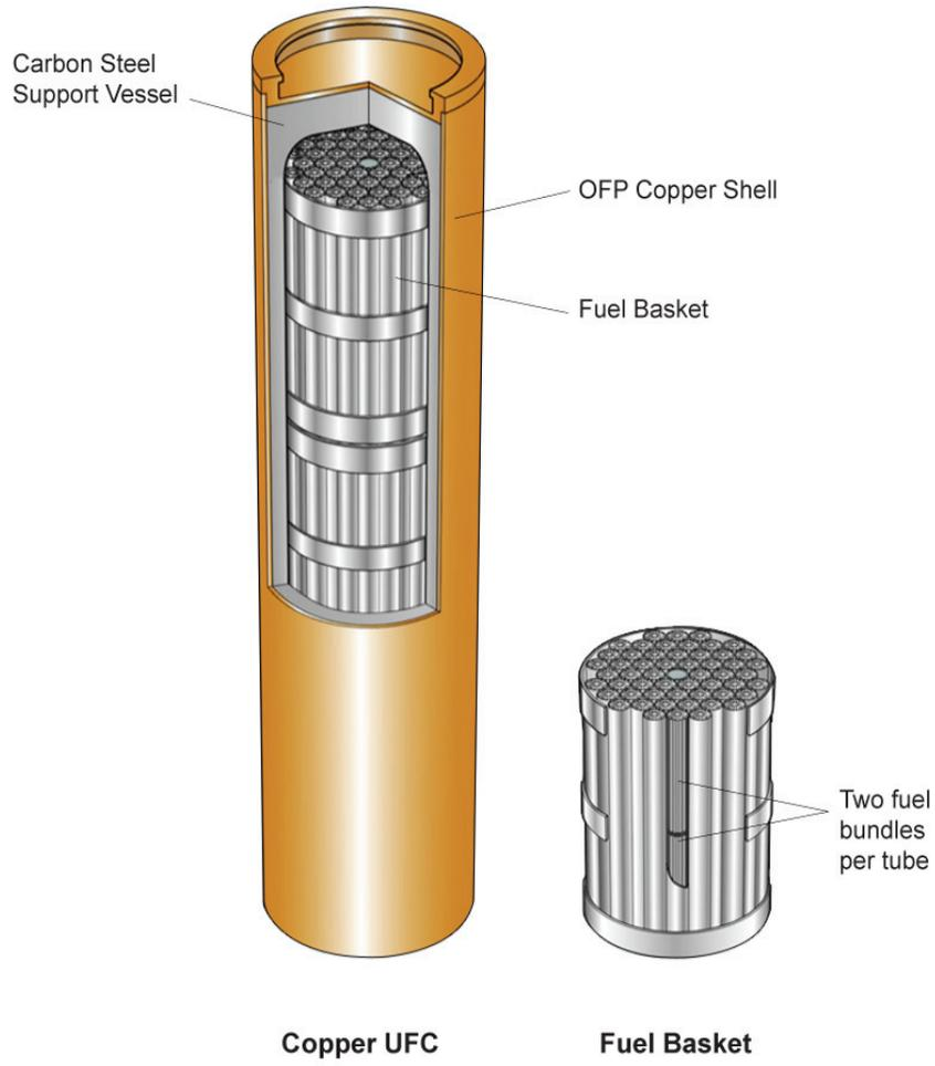
**Figure 4: Copper Used-fuel Container and Fuel Basket Holding Two Layers of CANDU Fuel Bundles**
