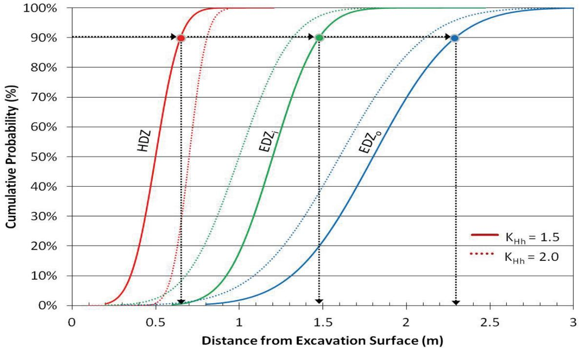
Figure 4.7: Cumulative Probability Distribution for Limestone Showing the EDZs for Both a Horizontal Stress Ratio of 1.5 and 2; the Arrows Indicate the Dimensions of the EDZs with 90% Confidence
