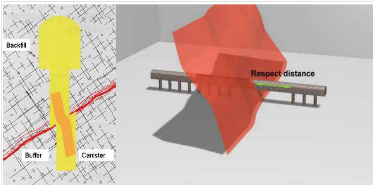
**Figure 4.9: Concept View of the Impact of a Fault-slip Event on a Waste Container in a Repository**
