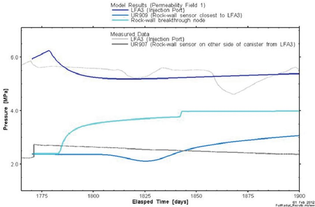
**Figure 5.2: Modelled Injection and Rock-Wall Pressures Using Heterogeneous Permeability Fields for LASGIT 2009 Gas Injection Test**
