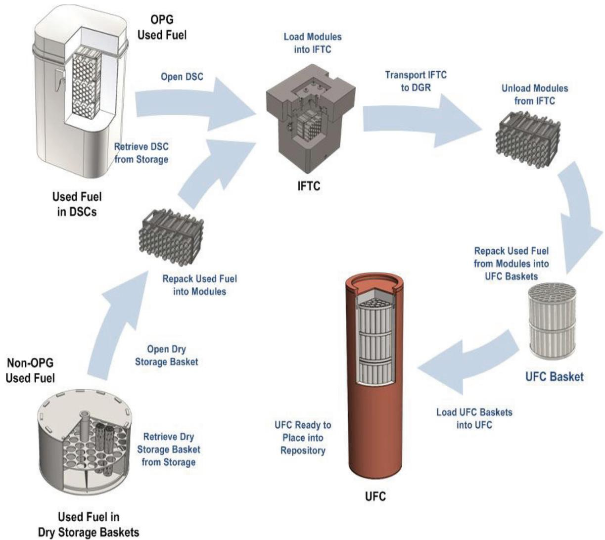
Figure 3.2: Flow Chart Illustrating a Process for Recovery and Transport of the Canadian Used Nuclear Fuel Stored at Reactor Sites; Dry Storage Container (DSC), UFC (Used Fuel Container), Irradiated Fuel Transfer Cask (IFTC)
