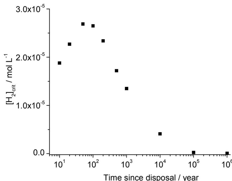
**Figure 5.1: Critical H<sub>2</sub> Concentration as a Function of Time after Disposal for CANDU Fuel with a Burnup of 220 MWh/kgU**
