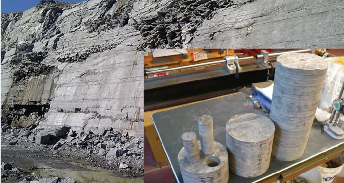
**Figure 4.1: Samples for THM Properties Collected at St Mary's Cement Quarry in Bowmanville, Ontario**
