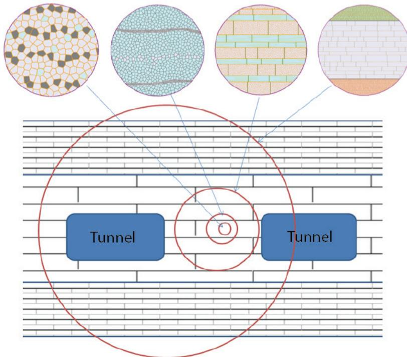
**Figure 4.3: Illustration Showing the Transition from Intact to a Bedded-jointed Rock Mass with Increasing Sample Size**
