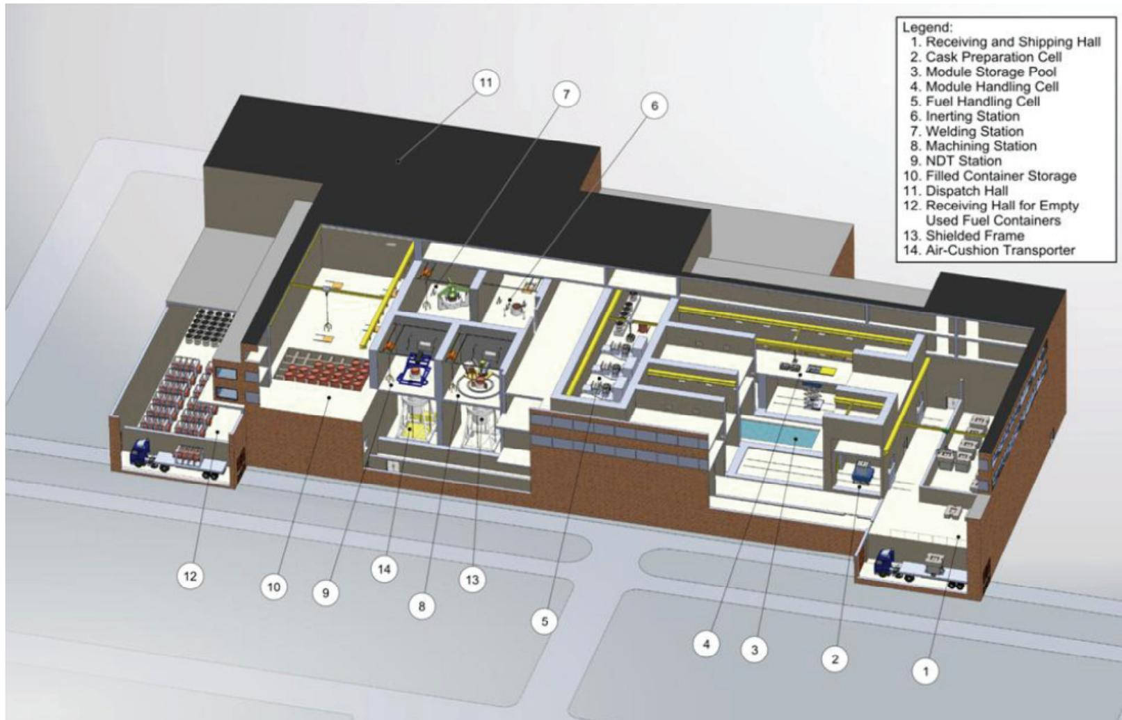
Figure 3.7: Design Concept for the Used Fuel Packing Plant
