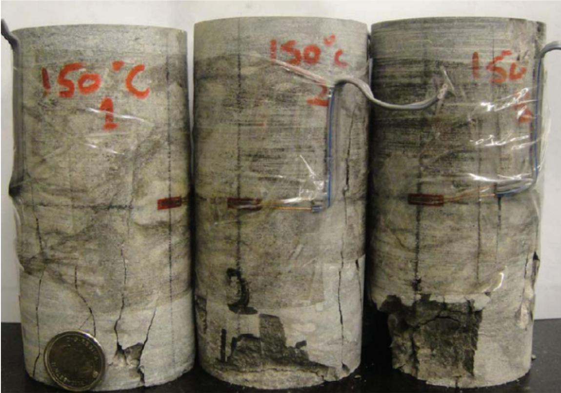
**Figure 4.2: Specimens Treated at 150°C, Following Completion of the Uniaxial Compressive Strength Test**
