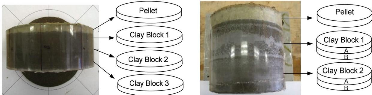
**Figure 3.9: Sampling Layers of Short (left) and Long (right) Specimens Surrounded by Plexiglas Sleeves**
