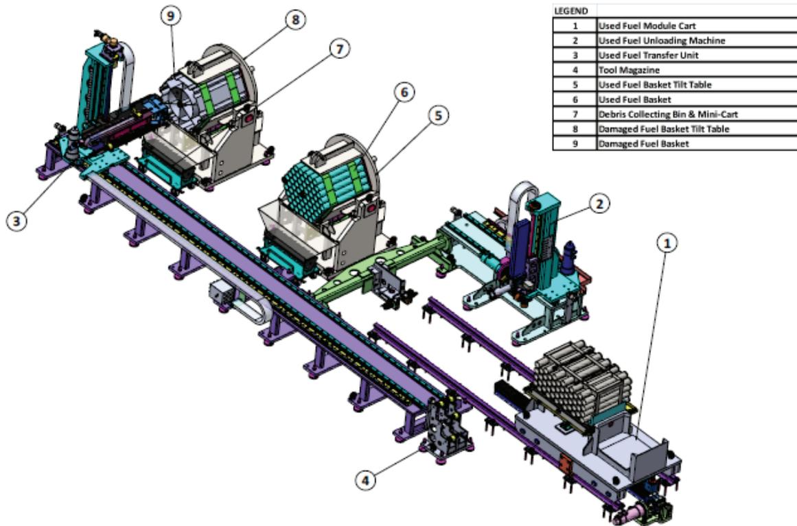
**Figure 3.8: Process and Equipment for the Transfer of Used Fuel from Storage Modules to UFC Baskets**
