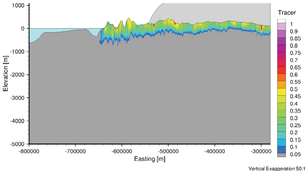
**Figure 4.11: Depth of Penetration for a Tracer of Unit Concentration Recharging from Surface during Glaciation**
