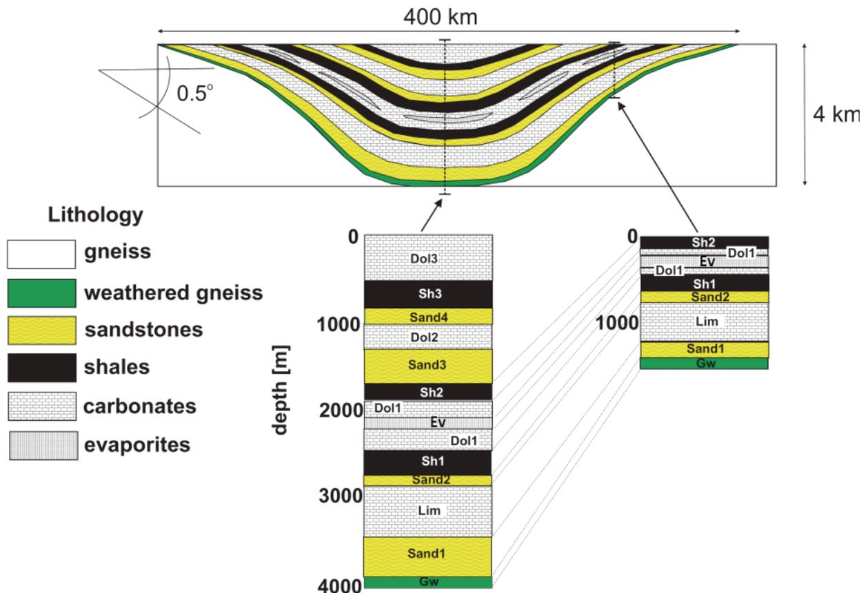
**Figure 4.12: Hypothetical Two-dimensional Sedimentary Basin for Modelling of Flow and Reactive Transport during a Single Glacial Cycle Using MIN3P-NWMO**
