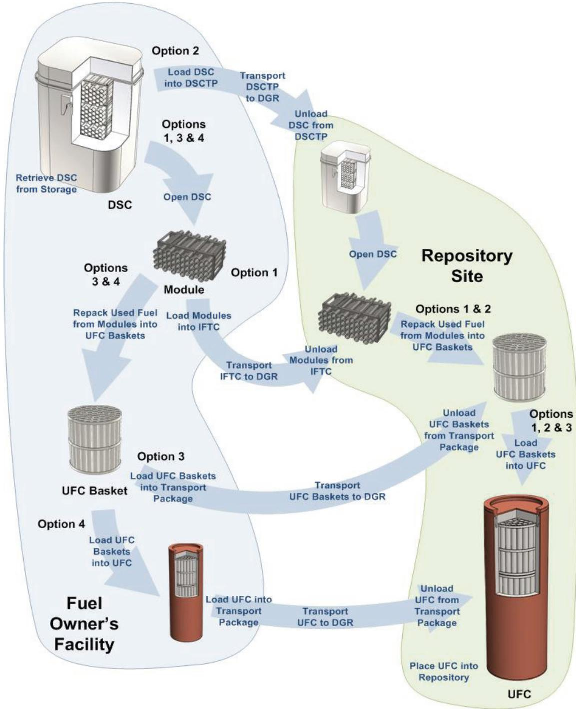
Figure 3.3: Flow Chart Showing Alternative Approaches to the Recovery of Used Fuel from Each Site and Transfer to the APM Facility; Dry Storage Container (DSC), Dry Storage Container Transport Package (DSCTP), UFC (Used Fuel Container), Irradiated Fuel Transfer Cask (IFTC)
