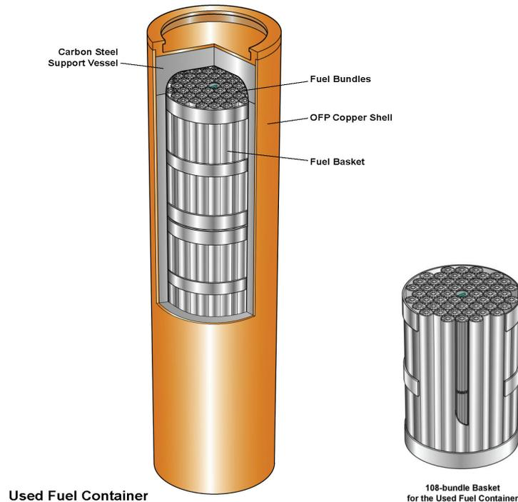
**Figure 3.4: Dual-Vessel Copper and Steel Used Fuel Container and Fuel Basket; Oxygen-Free Phosphorous-doped (OFP)**
