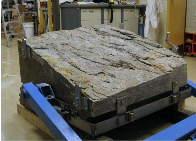
**Figure 4.10: View of the top surface of the fracture following separation of the Quarried Block.**
