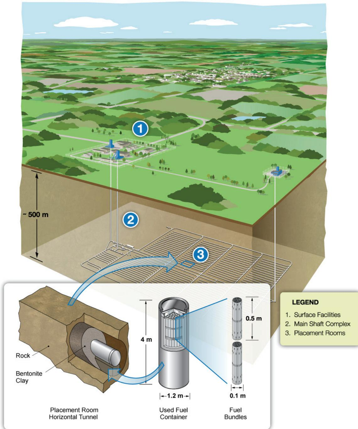
**Figure 2: Illustration of a reference deep geological repository (Steel used nuclear fuel container with horizontal tunnel placement) (Russell, 2011).**
