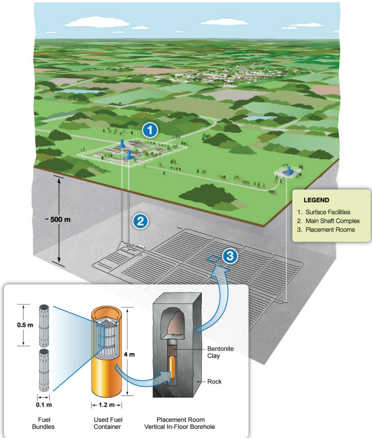
**Figure 1: Illustration of a reference deep geological repository (Copper-shell used nuclear fuel container with vertical in-floor borehole placement) (Russell, 2011).**
