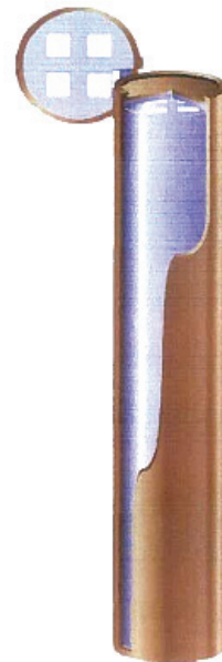
Figure 12: Similar Copper Used Fuel Container for High Burnup EPR fuel showing the container cross section after Raiko, 2005
