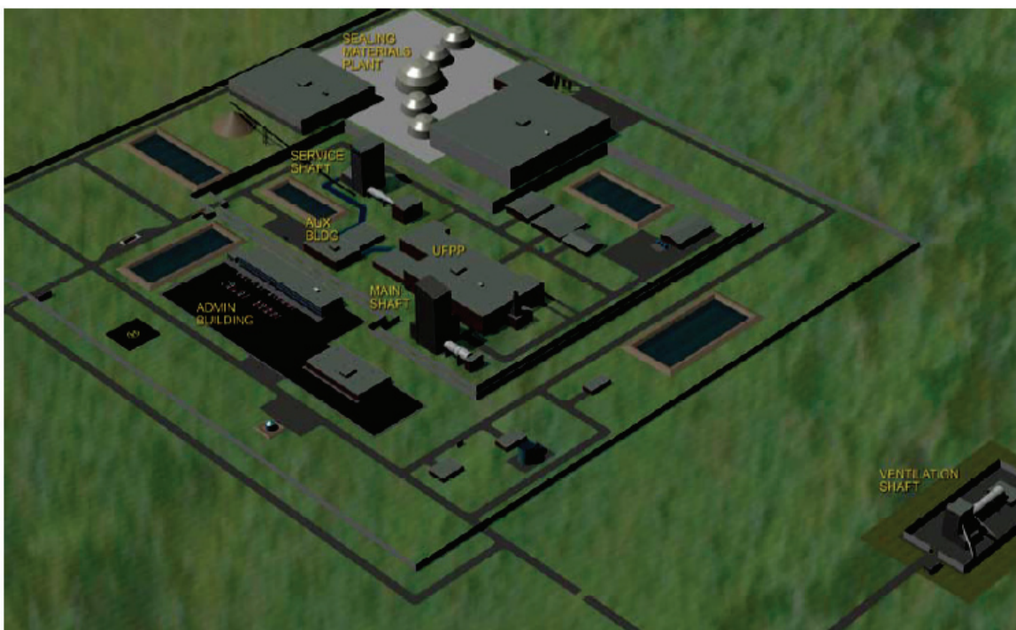
Figure 13: 3-D View of the DGR Surface Facilities, including the UFPP just north of the Main Shaft
