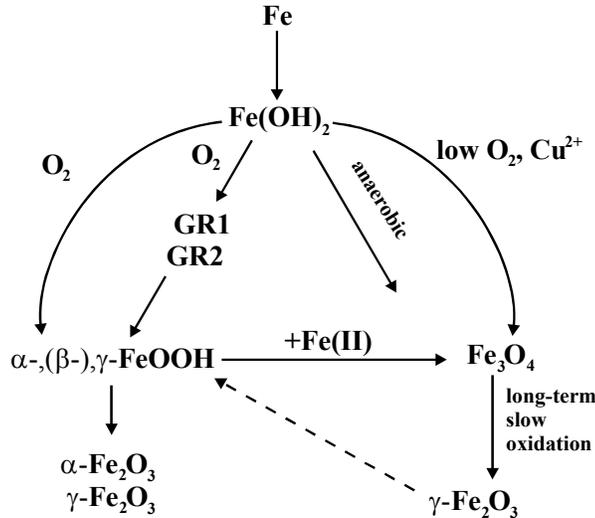
**Figure 3-3: Generalized Reaction Scheme for the Formation and Transformation of Corrosion Product Films on C-steel<sup>6</sup>**
