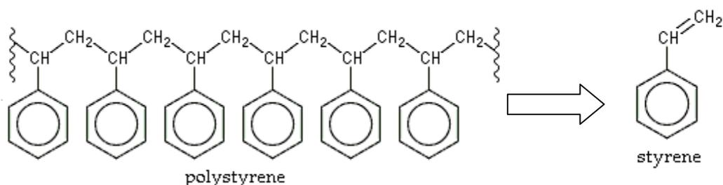
**Figure 3-2: Polystyrene Degradation**
