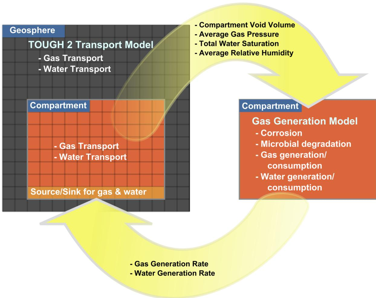
Figure 1-1: Coupling Gas Generation and Transport in T2GGM
