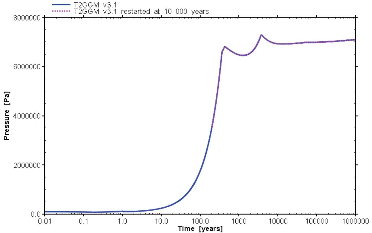
**Figure 5-8: Pressure in the GGM Container for 3DRS GG1 NWL Case, Comparing Version 3.1 and a Restart at 200 Years**
