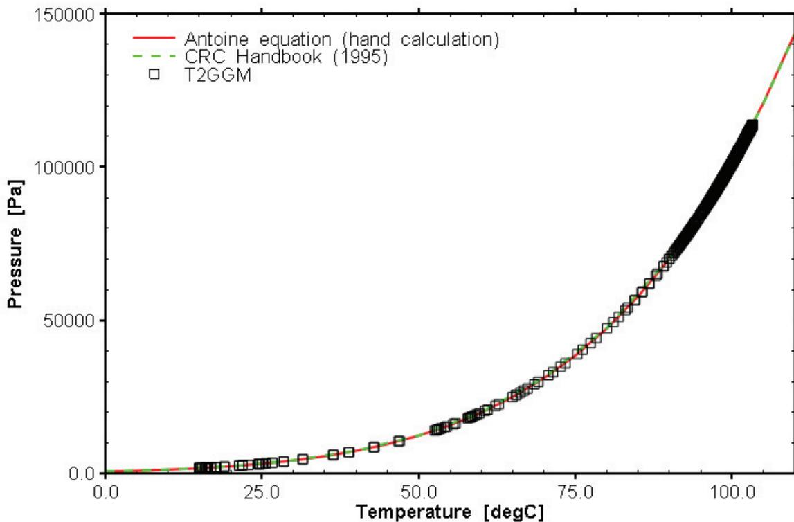
**Figure 5-2: Temperature-dependent Maximum Water Vapour Pressures as Calculated by T2GGM, Compared to Hand Calculations and Published Values**
