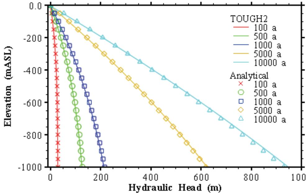
Figure 5-5: Analytical and T2GGM Calculated Hydraulic Head versus Depth at Different Times
