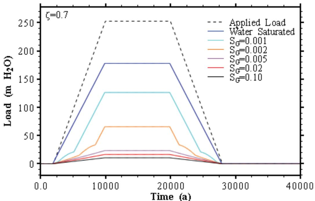
Figure 5-7: Effect of Gas Saturation
