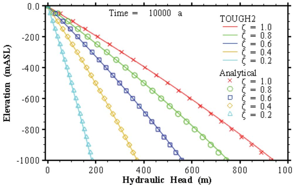
Figure 5-6: Analytical and T2GGM Calculated Hydraulic Head versus Depth at 10 000 years, for Different Loading Efficiencies ( $\zeta$ )
