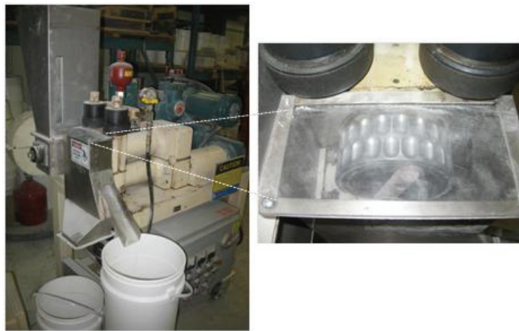
Figure 5: Laboratory- Scale Roller Compactor used in 2010 (Man et al. 2011) and 2011 Pellet Manufacturing Trials
