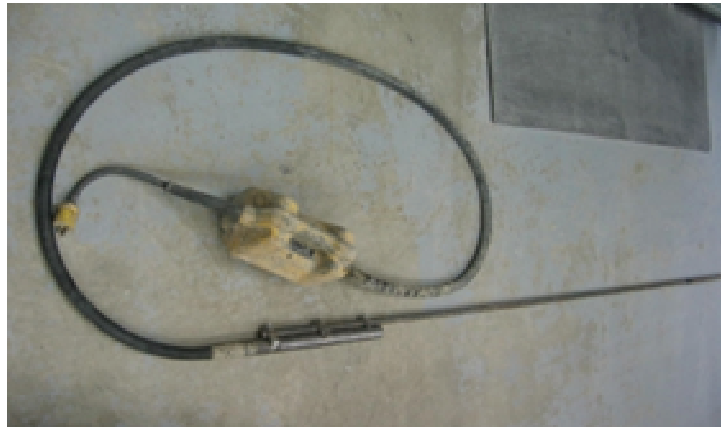
Figure 7: Rebar Shaker used to Aid in Pellet Fill Densification. The vibrating component is shown attached to a rebar in this photograph
