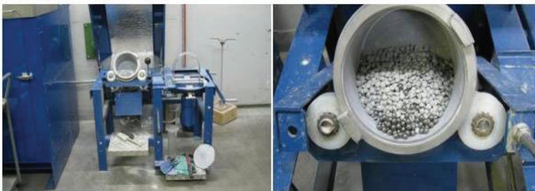
Micro-Deval test equipment
