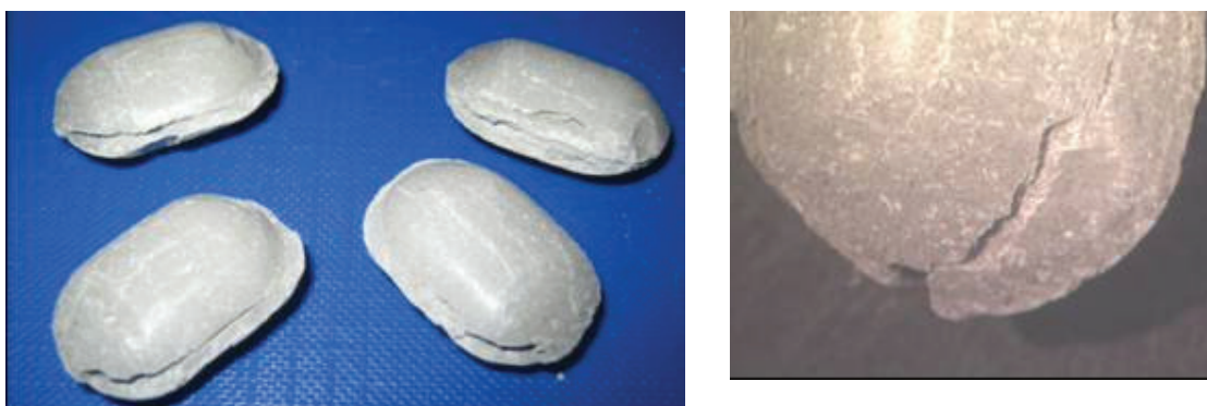
Figure 17: Visual Appearance of Large Pellets Exhibiting Surface Defects
