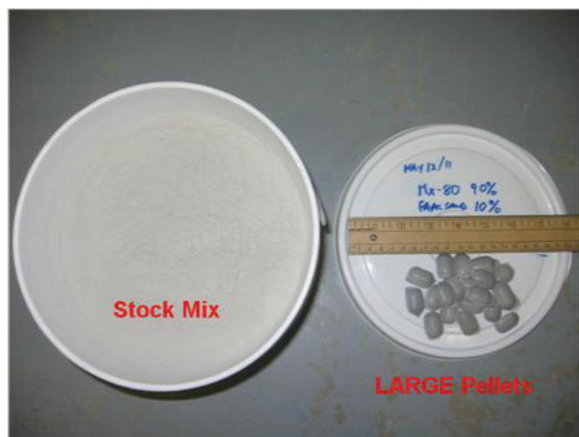
Figure 15: Colour Difference Between a Stock Mixture and Finished Pellets
