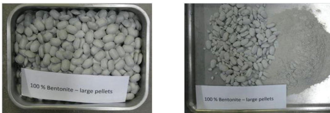
Large bentonite pellets tested for wear resistance, before (left) and after testing (right).
