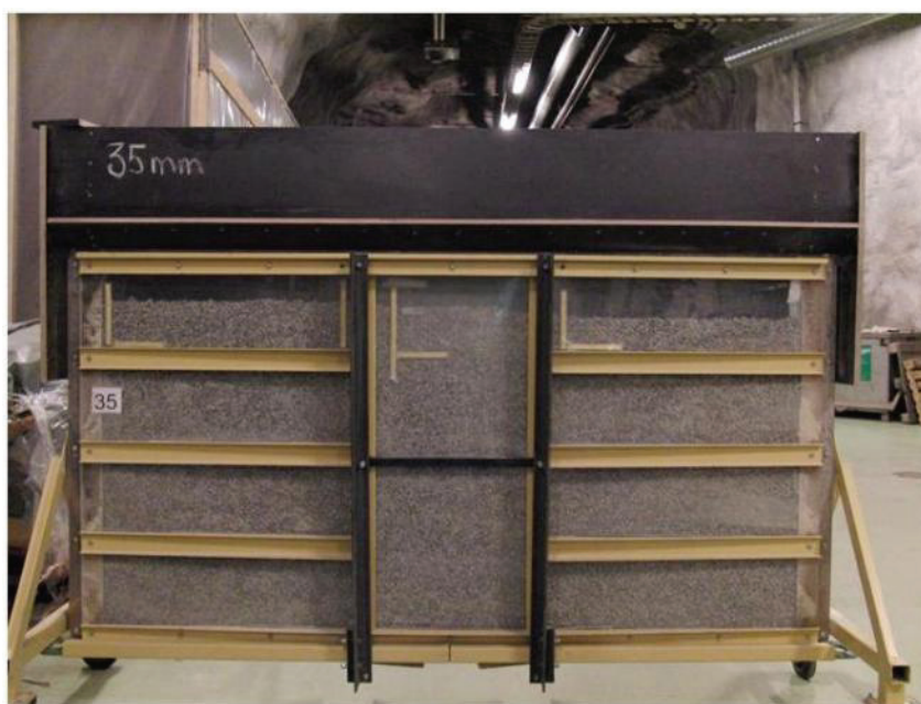
Figure 20: Large Pellet Pouring Test Frame at VTT
