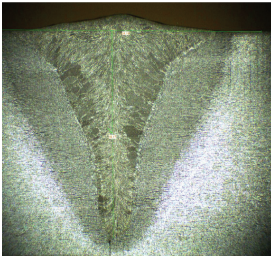
Figure 3.1: Macrograph Cross-section of a Typical 10 mm penetration Hybrid Laser Arc Weld Showing the Weld Fusion and Heat Affected Zone (5.6x magnification)
