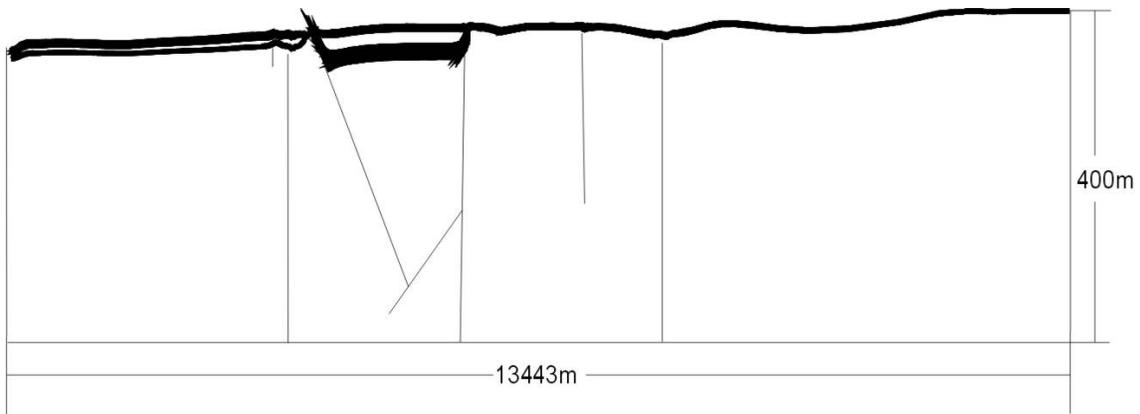
**Figure 39: Meltwater Recharge Paths Estimated by Tracking 137 Water-Coincident Particles Released into the Transient Flow Field Predicted by the 2D THM Simulation Using the Cold-based Glacial Scenario**
