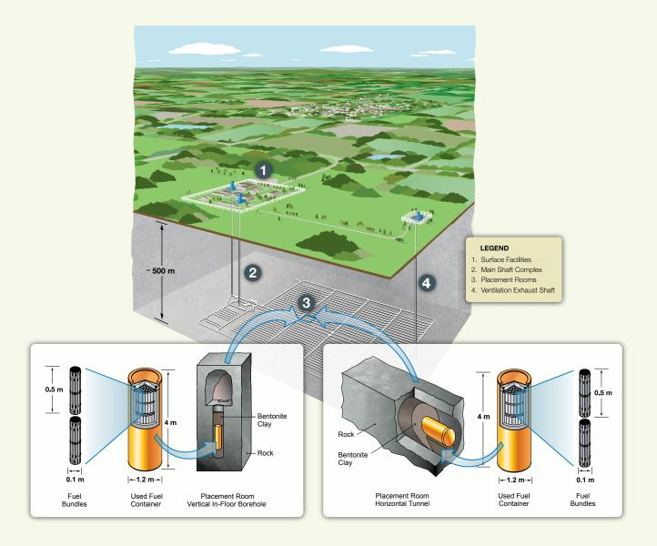
The containers will be placed in vertical boreholes drilled in the floor along the axis of a placement room, or placed horizontally within the confines of a placement room, depending on the nature of the rock and characteristics of the site.
