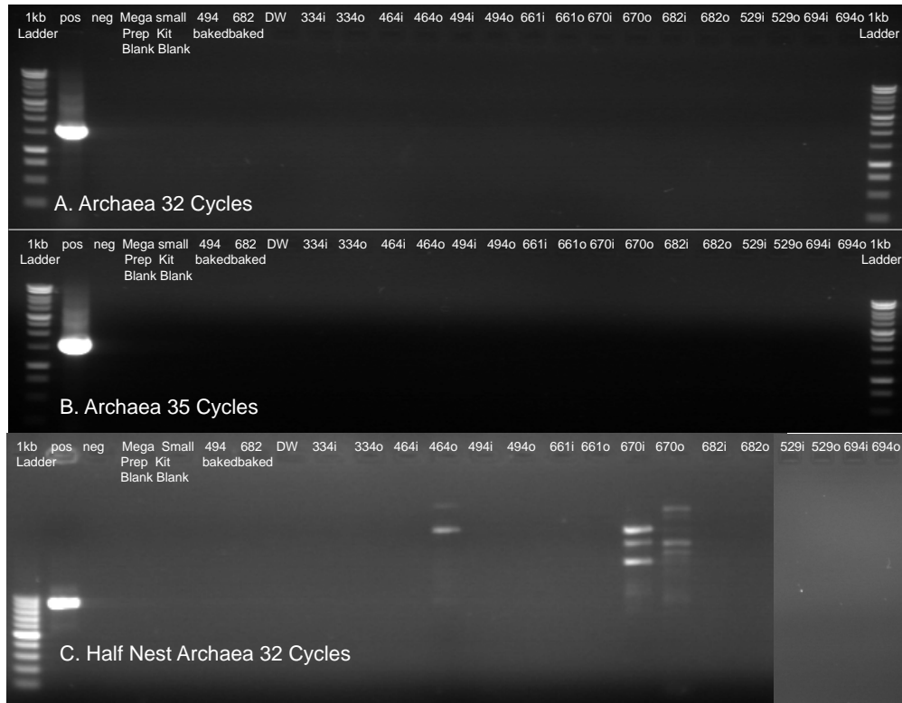
Figure 5: Stained Agarose Gel Illustrating Presence or Absence of Putative Archaeal PCR Products Under Conditions Tested: (A) 32 Cycles; (B) 35 Cycles; and (C) Half-nested reaction.
