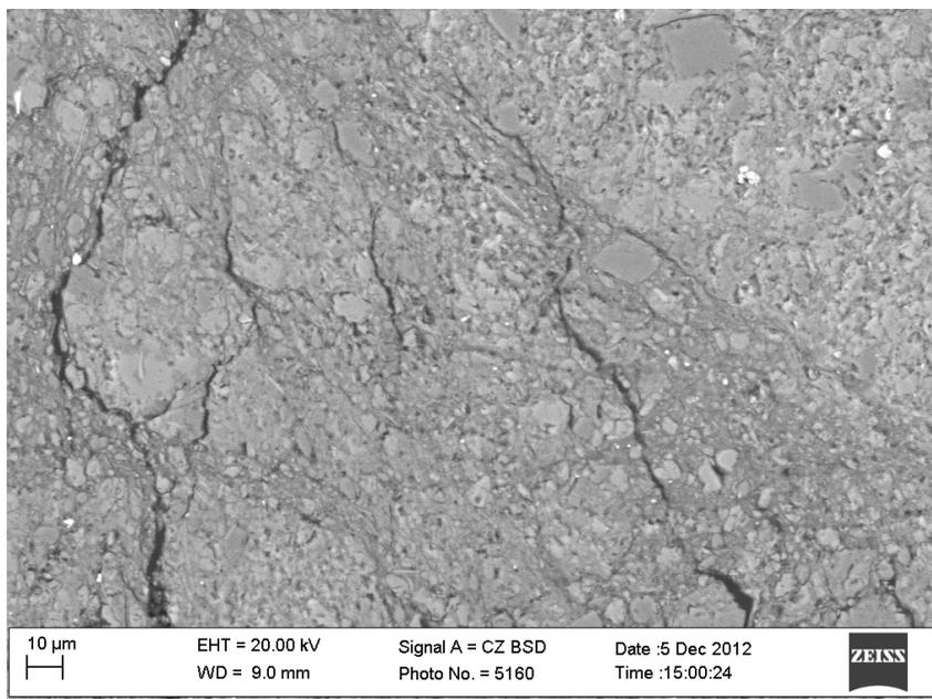
b.) Matrix destroyed due to fault gouge. Intact portion of the matrix in upper right corner
