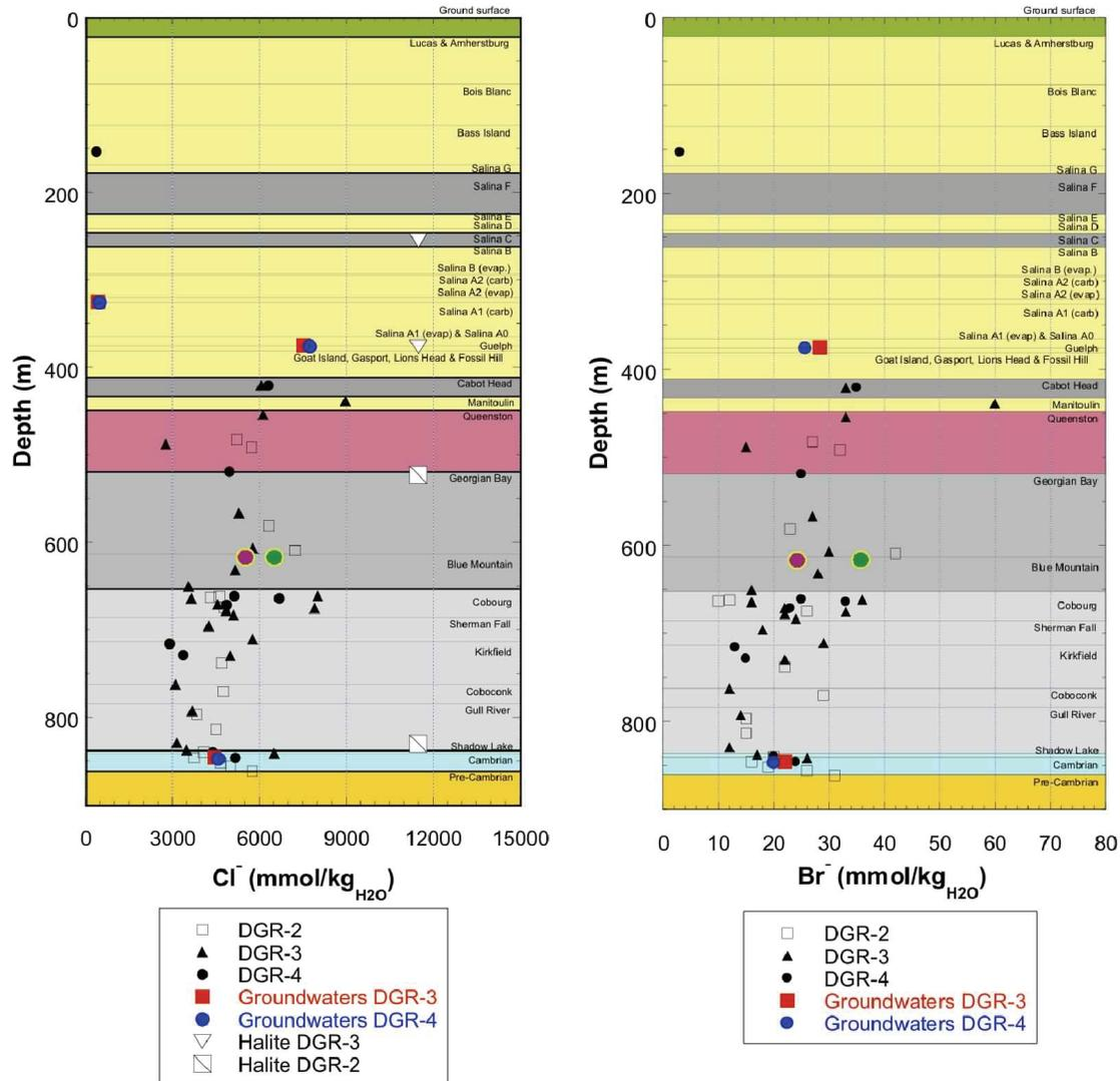
**Figure 20:  $\text{Cl}^-$  and  $\text{Br}^-$  Concentrations in Porewater of Sample DGR-4 610.48 Based on Squeezing (large green circle) and Aqueous Extraction (large purple circle) in Comparison With Pre-existing Aqueous Extraction Data of Hobbs et al. (2011); Adapted from Hobbs et al. (2011)**
