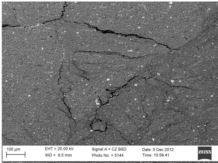
b.) Tectonised fabric with microfractures. Darker grey areas indicate destruction of the matrix fabric due to squeezing (formation of fault gouges). Bright area within microfracture in the upper left corner shows partial infill by halite
