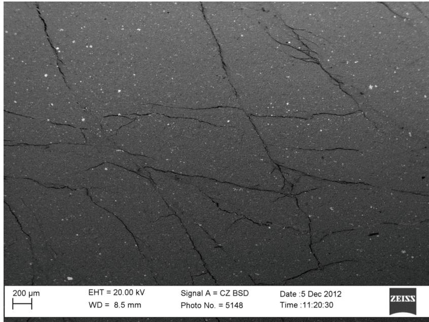
a.) Network of 2 sets of microfractures induced by squeezing
