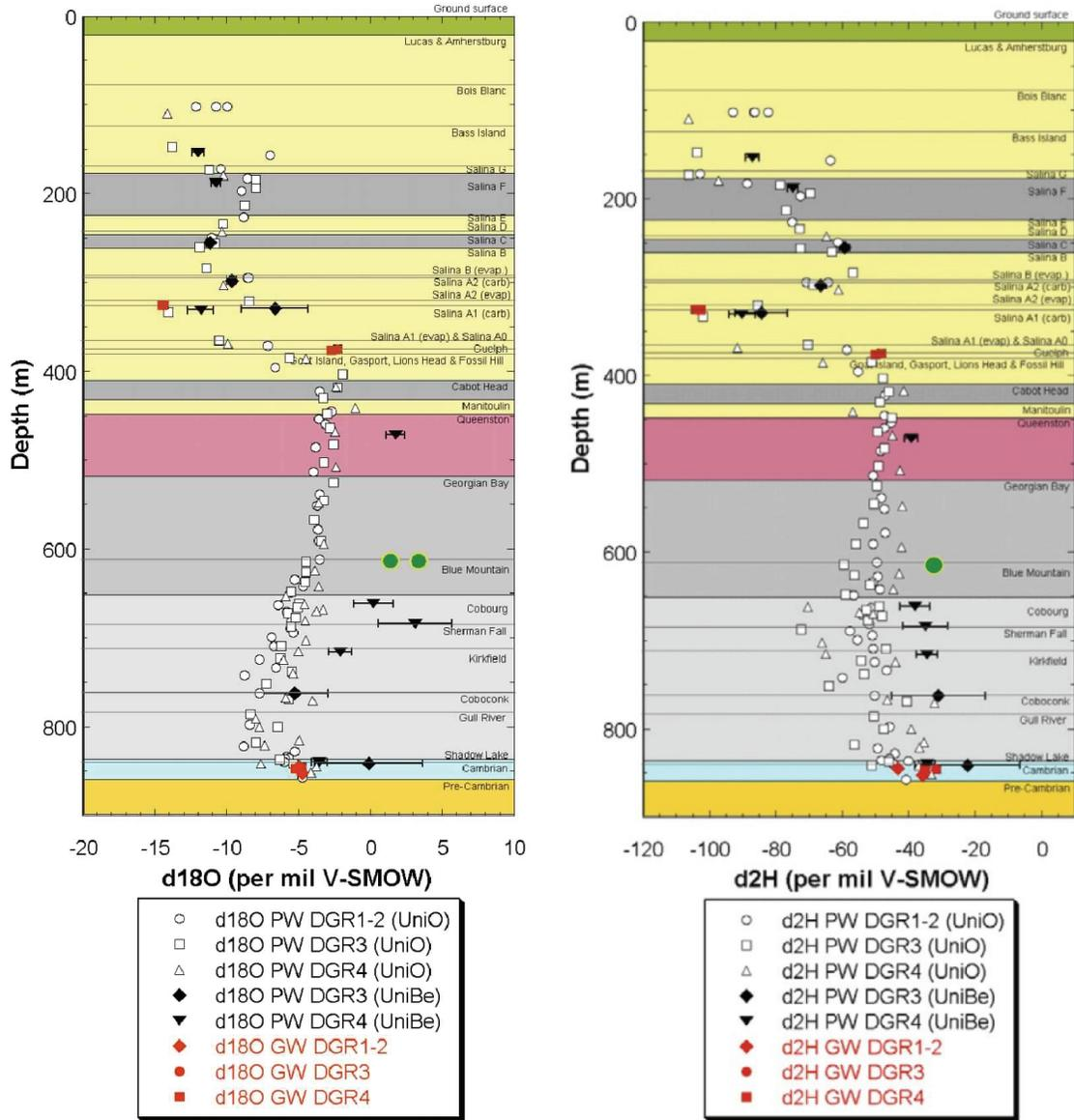
**Figure 26: Isotopic Composition of Porewater of Sample DGR-4 610.48 Based on Squeezing (large green circle) in Comparison With Pre-existing Aqueous Extraction Data of Hobbs et al. (2011) and Clark et al. (2010); Adapted from Hobbs et al. (2011)**
