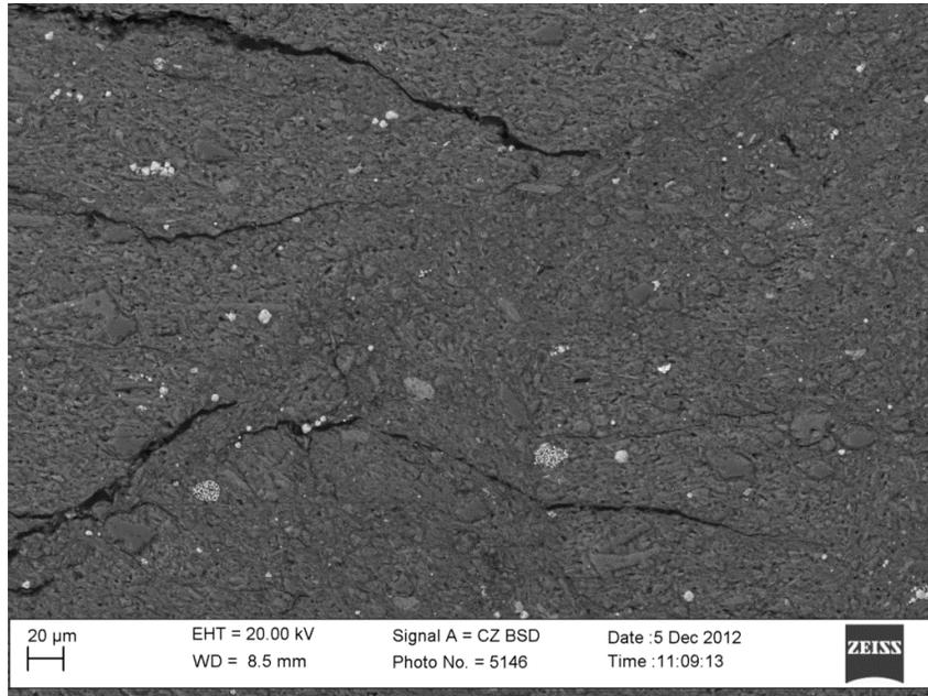
c.) Detail of b.). The lower right half of the image is a fault gouge
