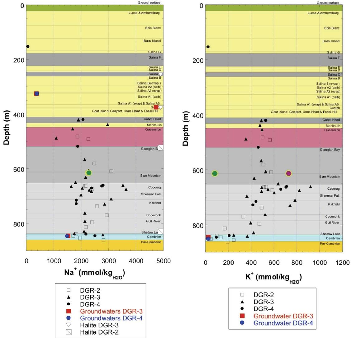
**Figure 22: Na<sup>+</sup> and K<sup>+</sup> Concentrations in Porewater of Sample DGR-4 610.48 Based on Squeezing (large green circle) and Aqueous Extraction (large purple circle) in Comparison With Pre-existing Aqueous Extraction Data of Hobbs et al. (2011); In Graph for Na<sup>+</sup>, the Point Obtained from Aqueous Extraction is Not Visible Because of a Complete Overlap With the Point from Squeezing; Adapted from Hobbs et al. (2011)**
