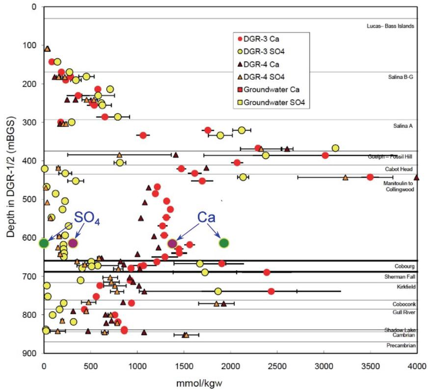
**Figure 25:  $\text{Ca}^{2+}$  and  $\text{SO}_4^{2-}$  Concentrations in Porewater of Sample DGR-4 610.48 Based on Squeezing (large green circle) and Aqueous Extraction (large purple circle) in Comparison With Pre-existing Aqueous Extraction Data of Clark et al. (2010); Adapted from Clark et al. (2010)**
