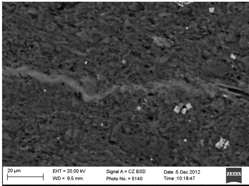
b.) Detail of a.). The halite infill is incomplete, some space remains open on the right side
