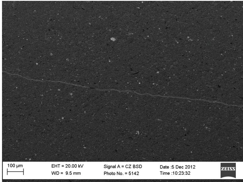
a.) Homogeneous, clay-rich rock matrix cross cut by a halite-filled microfracture (probably formed during sample drying)
