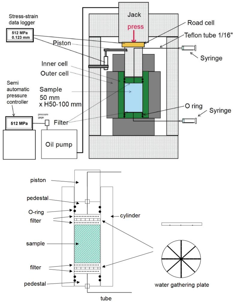
Figure 2: Rock Squeezing Apparatus at CRIEPI
