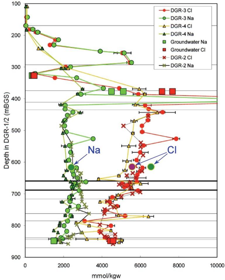
**Figure 21:  $\text{Na}^+$  and  $\text{Cl}^-$  Concentrations in Porewater of Sample DGR-4 610.48 Based on Squeezing (large green circle) and Aqueous Extraction (large purple circle - not visible because of a complete overlap with the point for  $\text{Na}^+$  from squeezing) in Comparison With Pre-existing Aqueous Extraction data of Clark et al. (2010); Adapted from Clark et al. (2010)**
