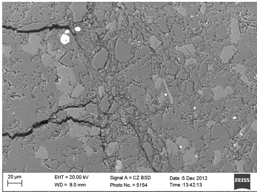
b.) Detail of a.) showing disintegration of rock fabric and grain-size reduction
