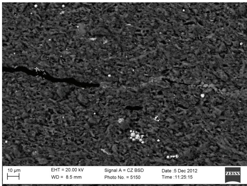
d.) Microfracture partially filled with halite
