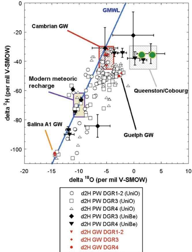
**Figure 27:  $\delta^{18}\text{O}$  vs.  $\delta^2\text{H}$  of Pore and Ground Waters from DGR Boreholes (compilation from Hobbs et al. 2011) and Data Points for the Squeezed Water from Sample DGR-4 610.48 (large green circles); Closed Black Symbols are Data based on Diffusive Exchange (University of Bern), Open Black Symbols are Data Based on Vacuum Distillation (University of Ottawa, Clark et al. 2010); Adapted from Hobbs et al. (2011)**
