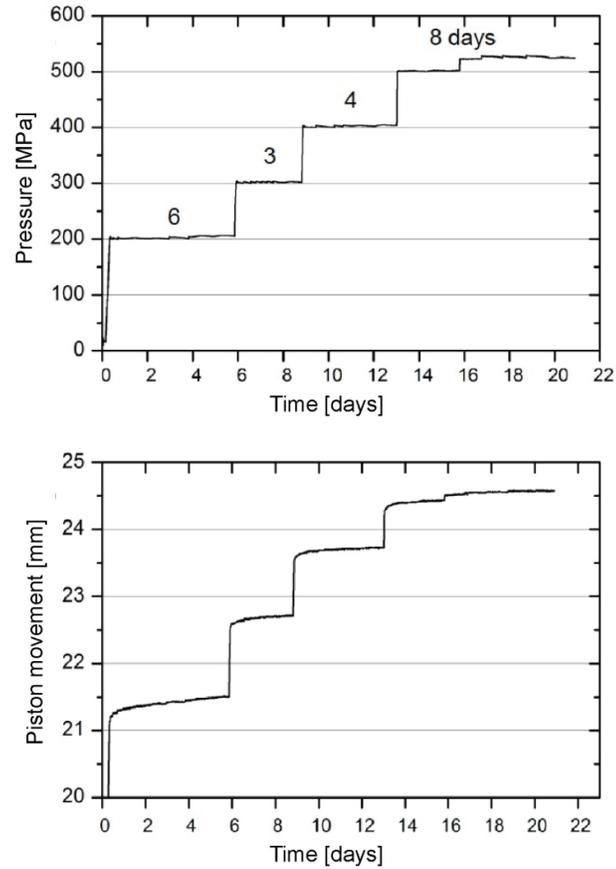
**Figure 5: Experiment With Sample DGR-4 610.48 I - Squeezing Pressure (top) and Piston Movement (bottom) as a Function of Time**
