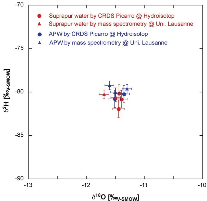
**Figure 19: Comparison of Isotope Analyses of APW and the Suprapur Water**
