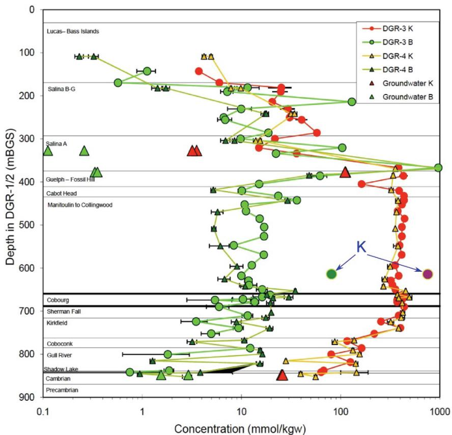
**Figure 23:  $K^+$  Concentration in Porewater of Sample DGR-4 610.48 Based on Squeezing (large green circle) and Aqueous Extraction (large purple circle) in Comparison With Pre-existing Aqueous Extraction Data of Clark et al. (2010); Adapted from Clark et al. (2010)**
