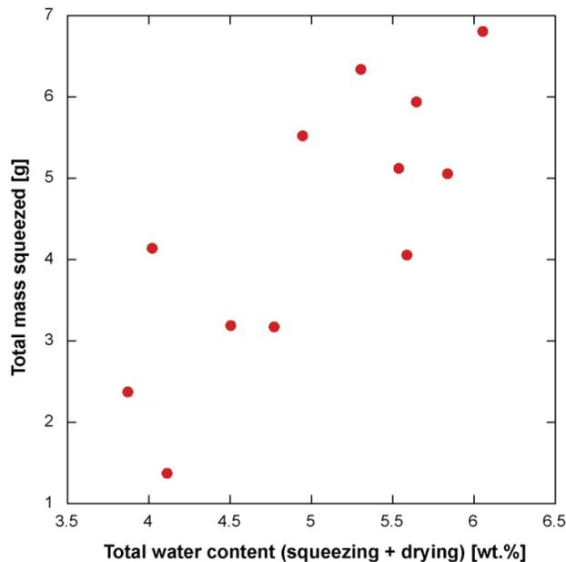
**Figure 1: Total Water Mass Squeezed as a Function of Water Content of Clay-rich Samples from the Mesozoic of the Schlattigen Borehole (from Wersin et al. 2013)**
