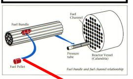
**Nuclear energy** is derived from uranium used in nuclear fission. Fuel bundles produce heat to create steam
