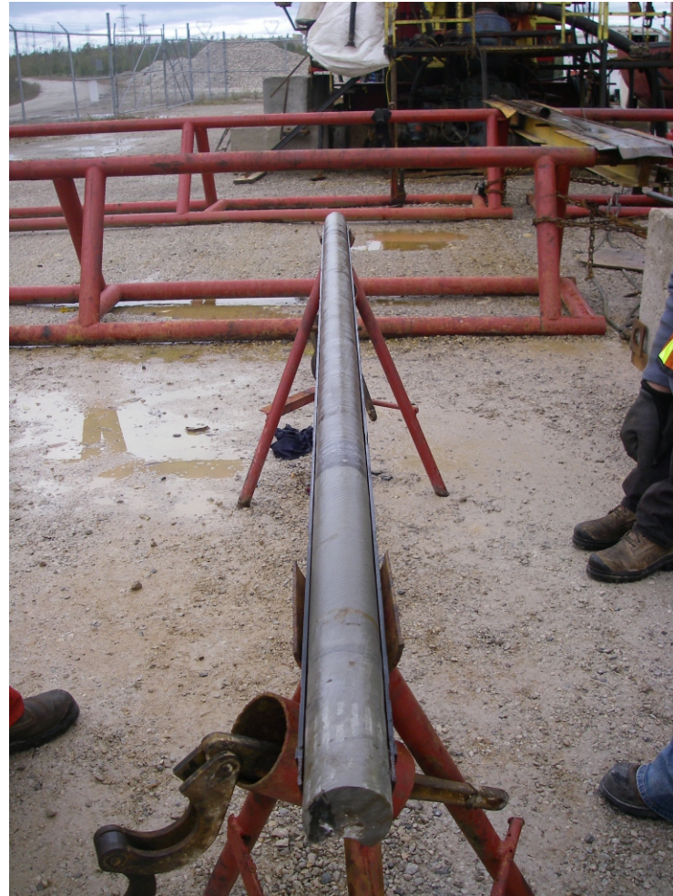
a. Manitoulin Formation Dolostone 480.75 - 483.79 mBGS in DGR-5
