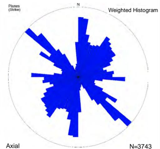
Length-weighted rose diagram of interpreted lineaments in the Manitowadge area
