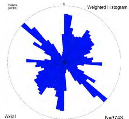
Length-weighted rose diagram of interpreted lineaments in the Manitowadge area
