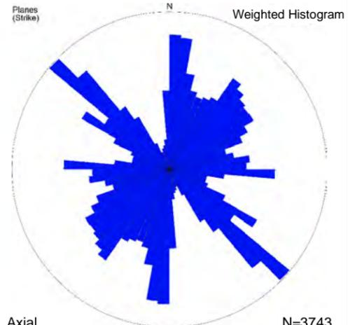
Axial Length-weighted rose diagram of interpreted lineaments in the Manitowadge area
