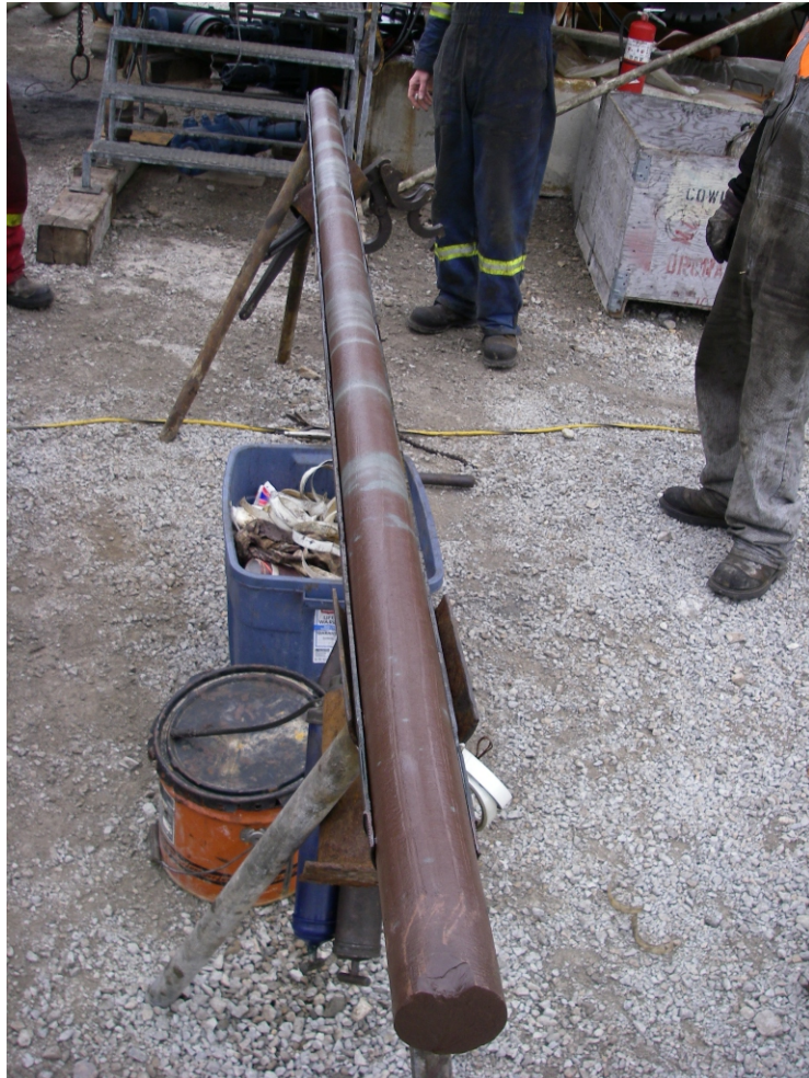
b. Queenston Formation Shale 475.73 - 478.78 mBGS in DGR-3
