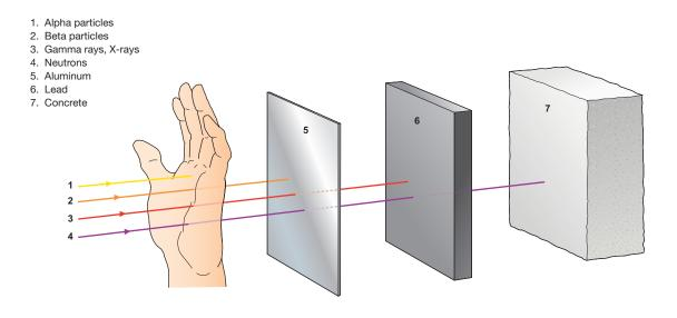
As shown, alpha particles and low energy beta particles cannot penetrate human skin. Beta particles can penetrate human skin, but skin is easily shielded from beta particles by a thin aluminum foil. Higher energy radiation – such as neutrons, gamma rays, and x-rays – can penetrate skin, but can be stopped by lead or concrete shielding.
