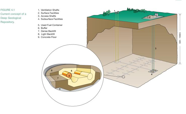
In the AECL disposal concept (the specific concept referred to in the Act), multiple barriers are proposed for limiting such movement. Barriers include:
