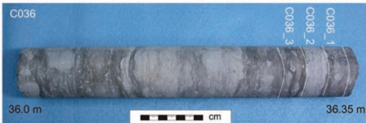
Figure 1: Drill core samples of Queenston Formation shale and Cobourg Formation limestone used for testing diffusion measurements. The location of the diffusion test samples (C036_1 to C036_3) is indicated on the Cobourg Formation core.
