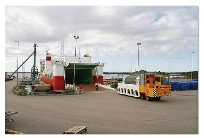
**Figure 8: Loading/unloading of radioactive waste onto SKB's m/s Sigyn in Sweden** (Source: SKB; Photographer: Bengt O Nordin)
