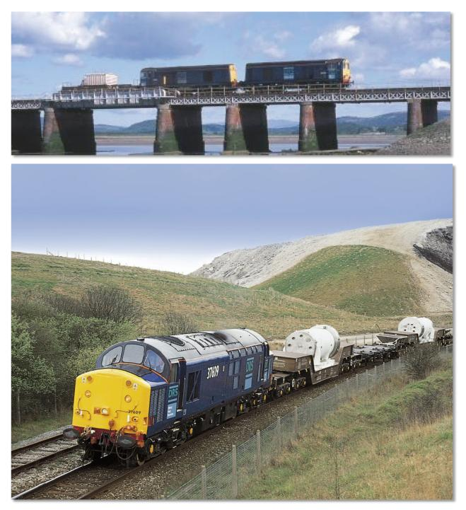
Figure 5: Trains carrying used nuclear fuel en-route to Sellafield (Source: Direct Rail Services)
