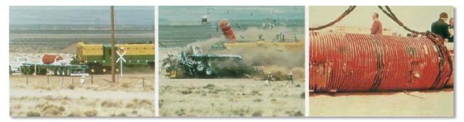
Figure 13: A Type B transportation cask being broadsided by a Locomotive in tests in USA (Source: DOE)
