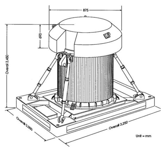
Figure A2: Isometric sketch of Pegase Cask (Source: US DOE)
