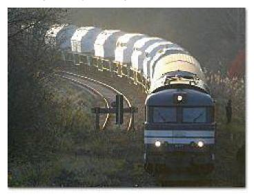
Figure 6: A typical train carrying used nuclear fuel in CASTOR casks between France and Germany (Source: de.indymedia.org)
