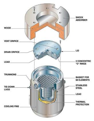
**Figure 12: A typical Type B used nuclear fuel transportation cask (TN-TMR)** (Source: Transnucleaire)
