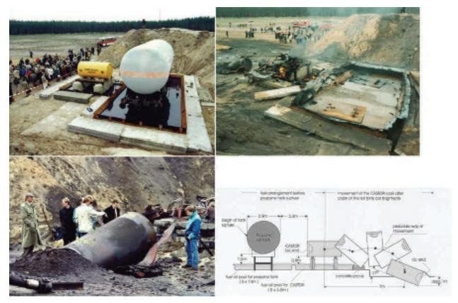
Figure 14: A Type B transportation cask struck by an exploding propane tank in a test in Germany (Source: BAM)
