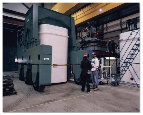
Figure A8: On-site movement of a Dry Storage Container (Source: OPG)
