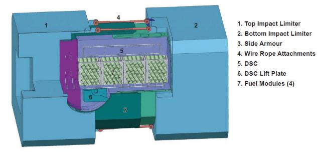
**Figure A7: Cut-away Sketch of the Dry Storage Container Transportation Package** (Source: OPG / NWMO)
