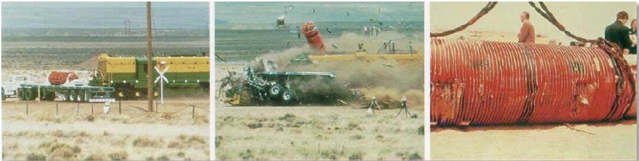
**Figure 13: A Type B transportation cask being broadsided by a Locomotive in tests in USA** (Source: DOE)
