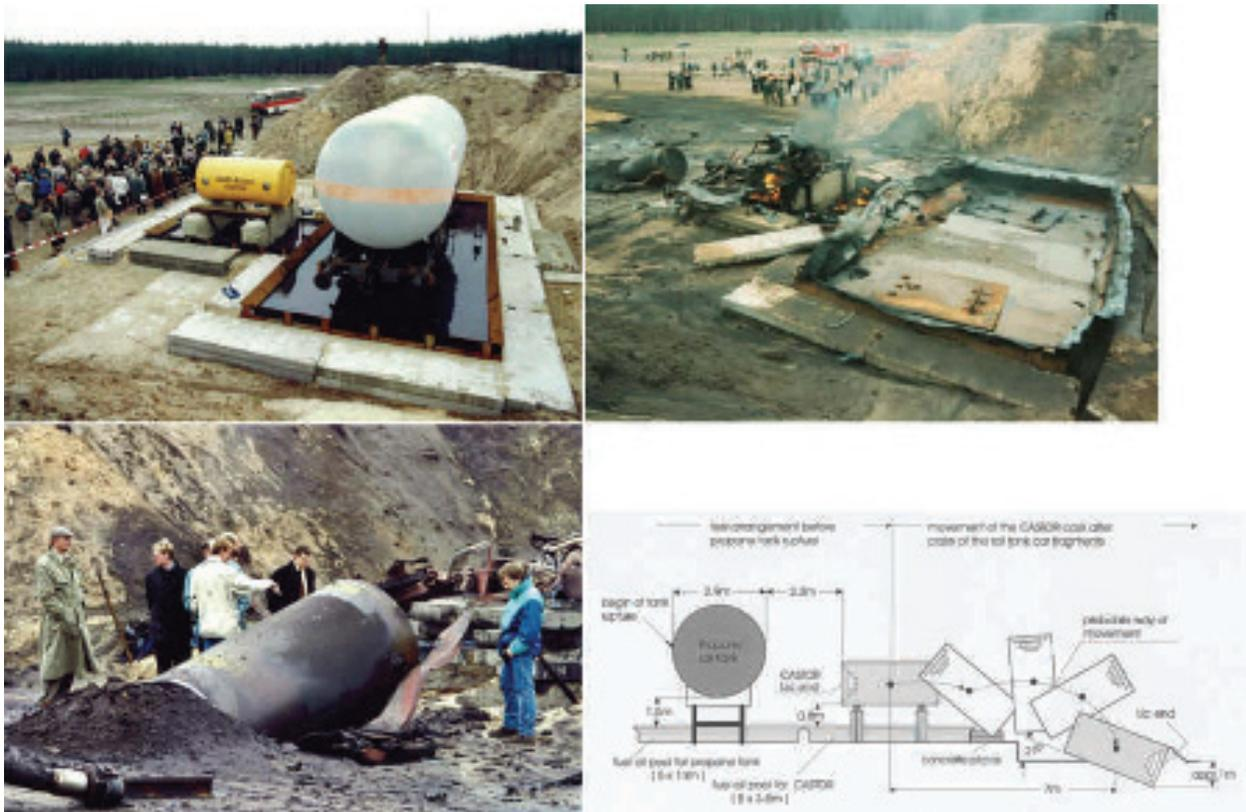
**Figure 14: A Type B transportation cask struck by an exploding propane tank in a test in Germany (Source: BAM)**
