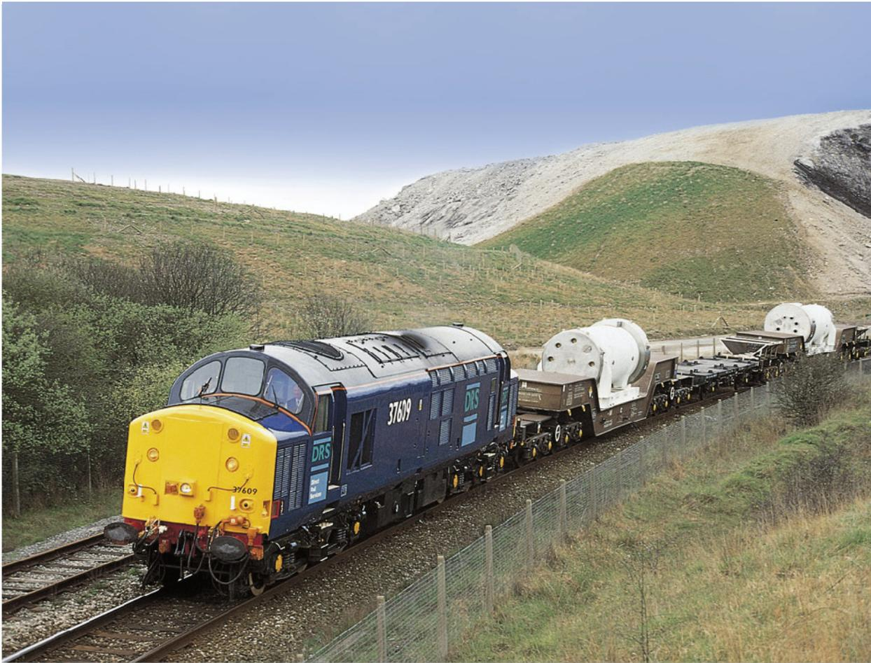
**Figure 5: Trains carrying used nuclear fuel en-route to Sellafield (Source: Direct Rail Services)**
