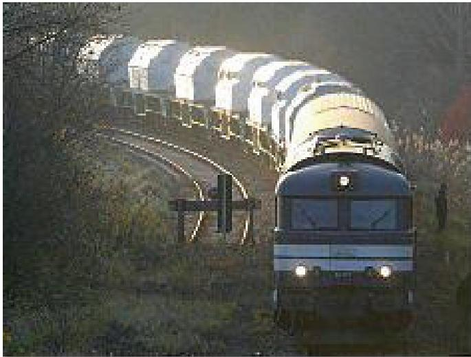
**Figure 6: A typical train carrying used nuclear fuel in CASTOR casks between France and Germany (Source: de.indymedia.org)**
