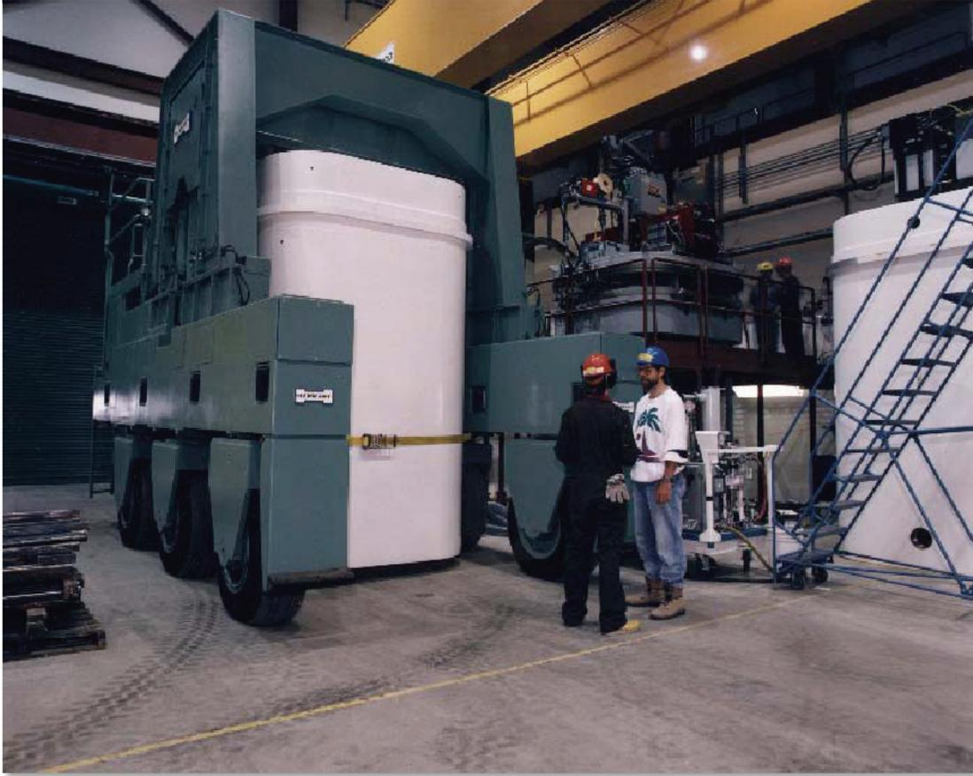
**Figure A8: On-site movement of a Dry Storage Container (Source: OPG)**
