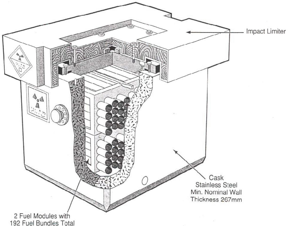
**Figure A5: Isometric Sketch of the Irradiated Fuel Cask (Source: OPG / NWMO)**
