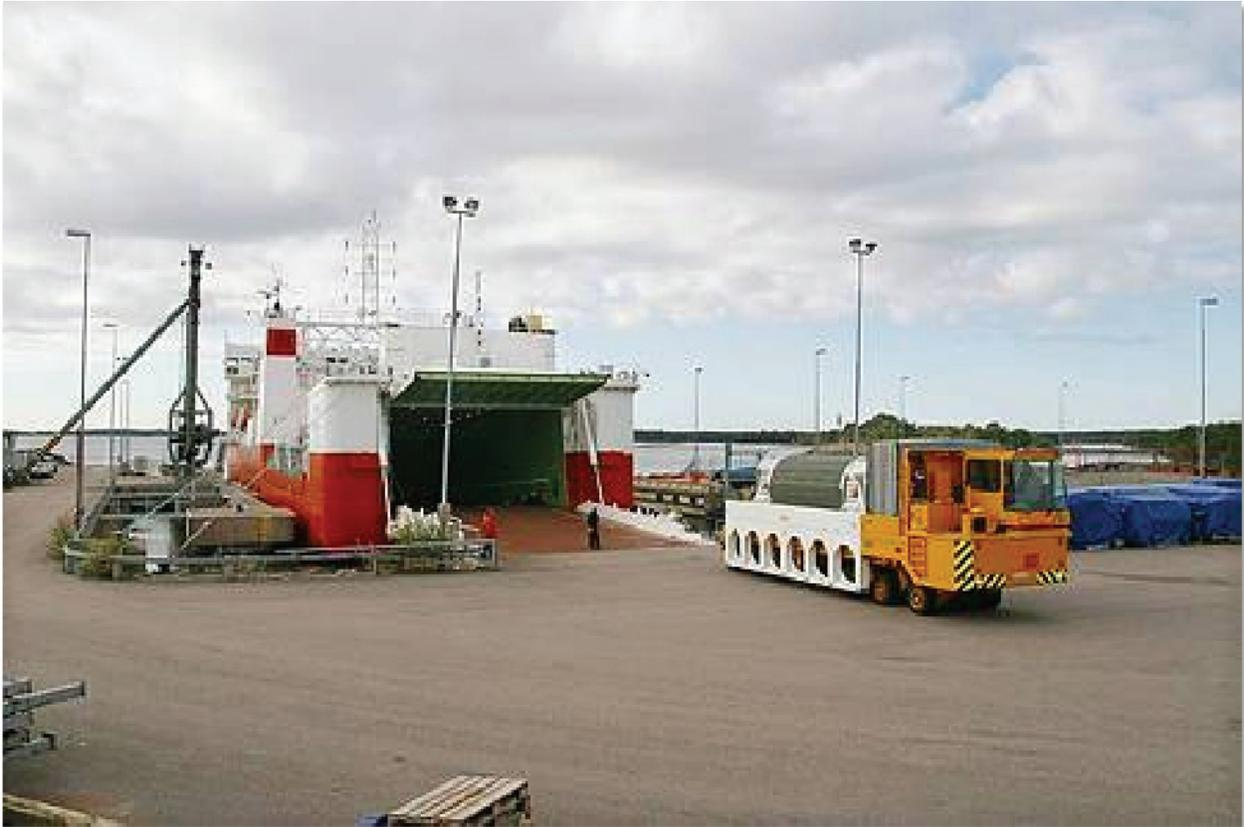
**Figure 8: Loading/unloading of radioactive waste onto SKB's m/s Sigyn in Sweden**
