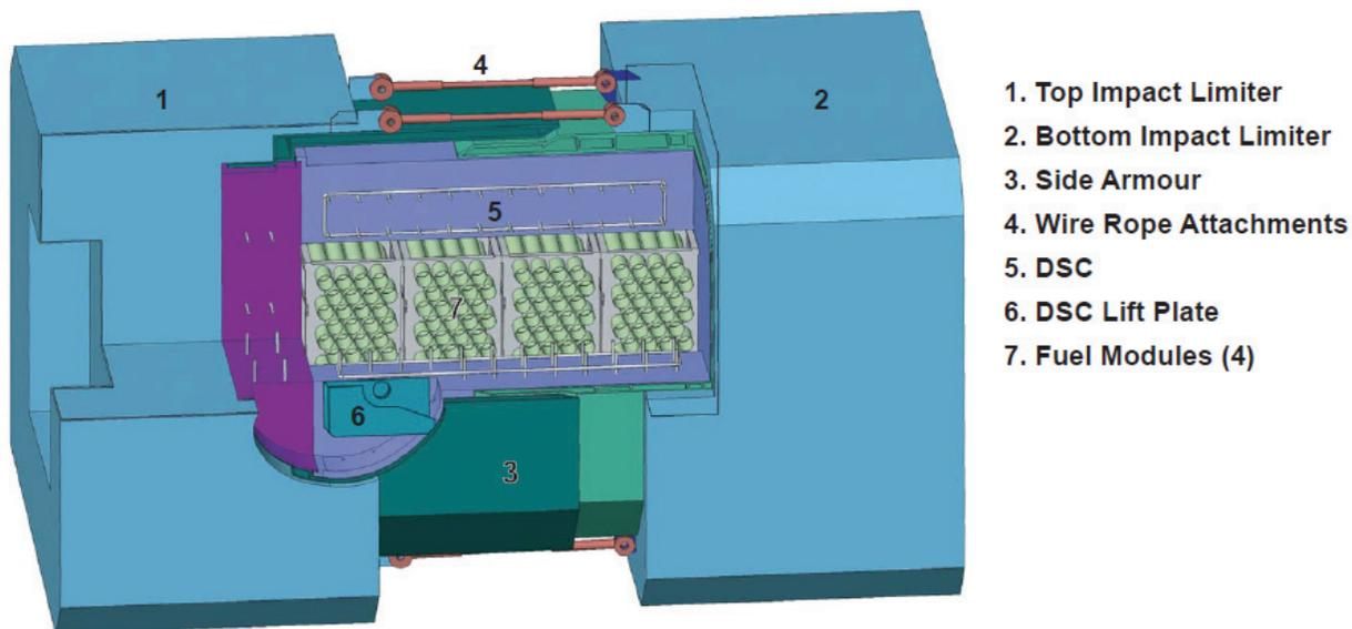
**Figure A7: Cut-away Sketch of the Dry Storage Container Transportation Package**
