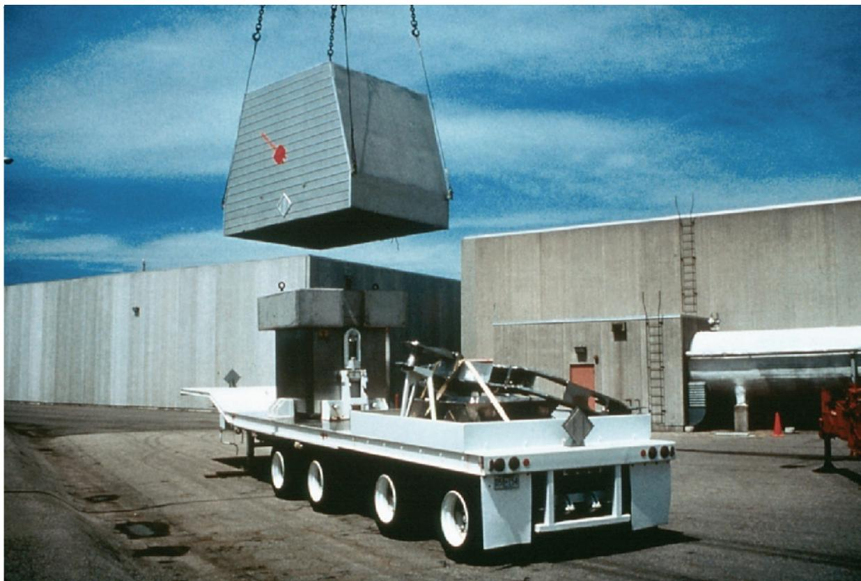
**Figure A6: Photo of Ontario Power Generation's Irradiated Fuel Cask on trailer (Source: OPG / NWMO)**
