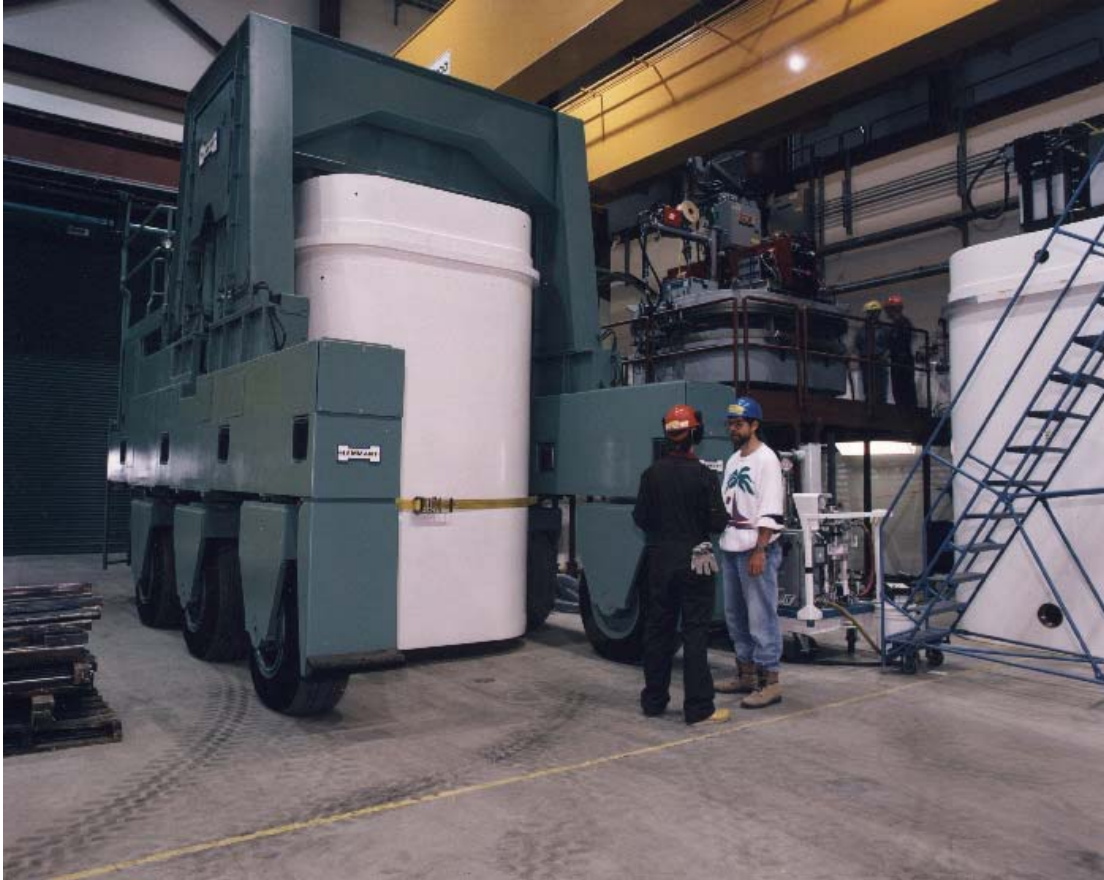
Figure D-4. Dry storage container and transporter (OPG).
