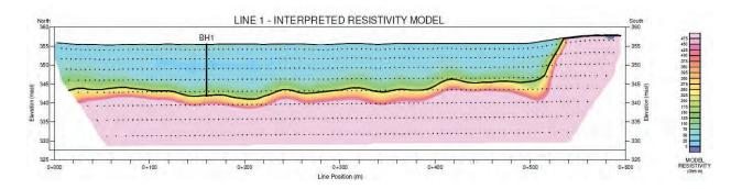
Figure 6-4: Example ERI model section showing the inferred upper bedrock surface overlain by silt and clay soils. (Golder Associates Ltd.)
