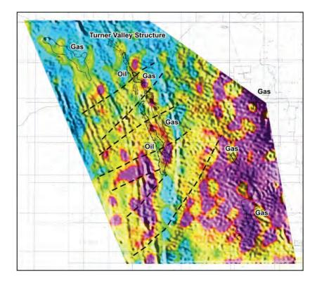
Figure 4-13: Airborne gravity survey example from Turner Valley, Alberta, Canada. (Sander Geophysics Ltd.)
