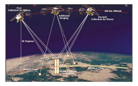
Figure 3-2: Satellite imagery acquisition. (GeoEye Inc.)
