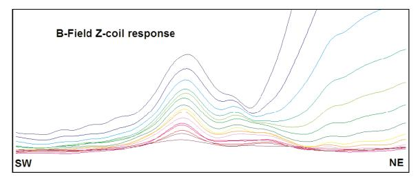
Figure 4-11: TDEM response over an inclined conductive target. (Fugro Airborne Surveys)
