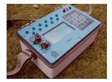
Figure 6-8: Elec Pro 10-channel IP Receiver (TerraPlus Inc.)
