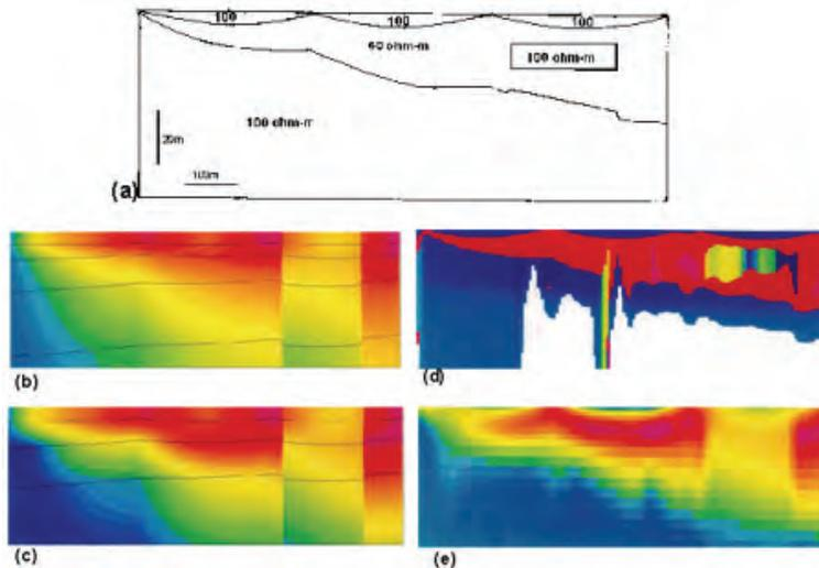
**Figure 4-12: An example of frequency domain EM inversion results. (Fugro Airborne Surveys)**
