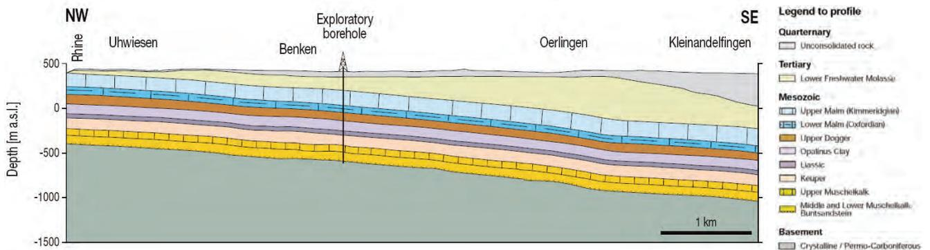
**Figure 7-11: A geological profile through Zürcher Weinland showing the major geologic units. (NAGRA, 2000)**
