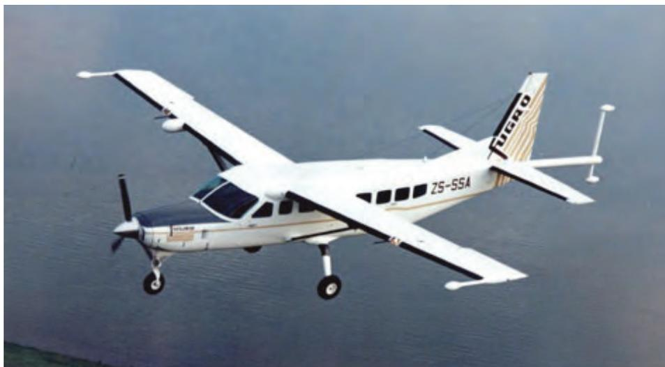
**Figure 4-5: A fixed wing aircraft mounted tri-axial gradient magnetic survey. (Fugro Airborne Surveys)**
