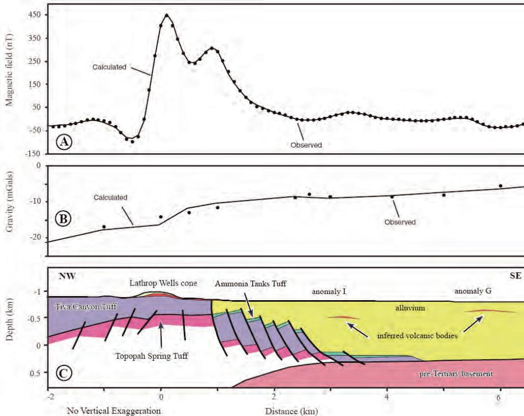
**Figure 7-8: Geophysical models showing fits between observed and calculated (A) magnetic and (B) gravity profiles and (C) a geologic interpretation of inferred subsurface structure at Yucca Mountain. Note the anomalies I and G, which are inferred to be basaltic volcanic bodies. (O’Leary et al., 2002)**
