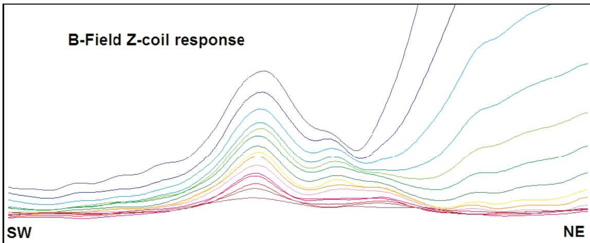
**Figure 4-11: TDEM response over an inclined conductive target. (Fugro Airborne Surveys)**
