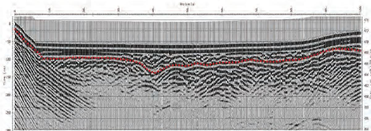
**Figure 6-6: Example 50 MHz GPR data used to map the top of bedrock. (Golder Associates Ltd.)**
