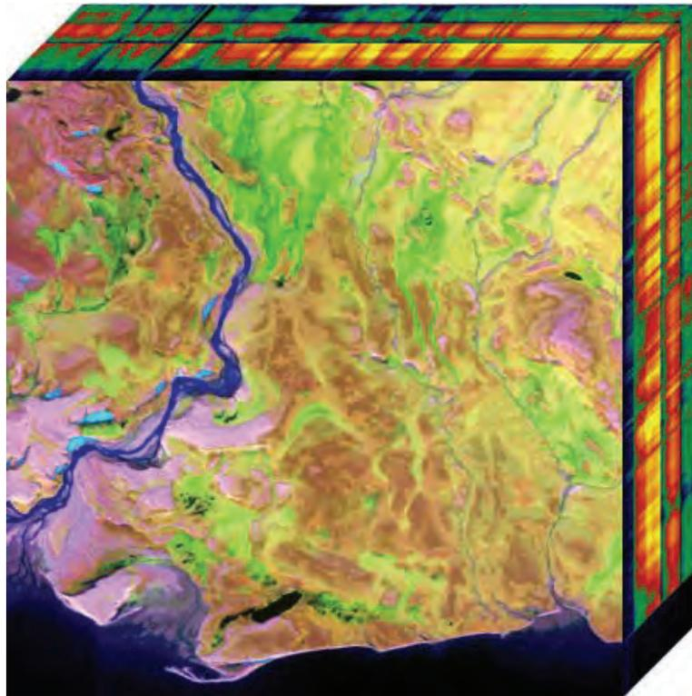
**Figure 4-4: A hyperspectral data cube example (Nicholas M. Short, Sr., June 18, 2007. The Remote Sensing Tutorial)**
