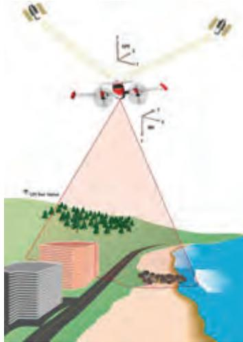
**Figure 4-2: Airborne LiDAR mapping illustrating LiDAR swath, orientation deviations, and aircraft receiving GPS signals. (Optech Inc.)**
