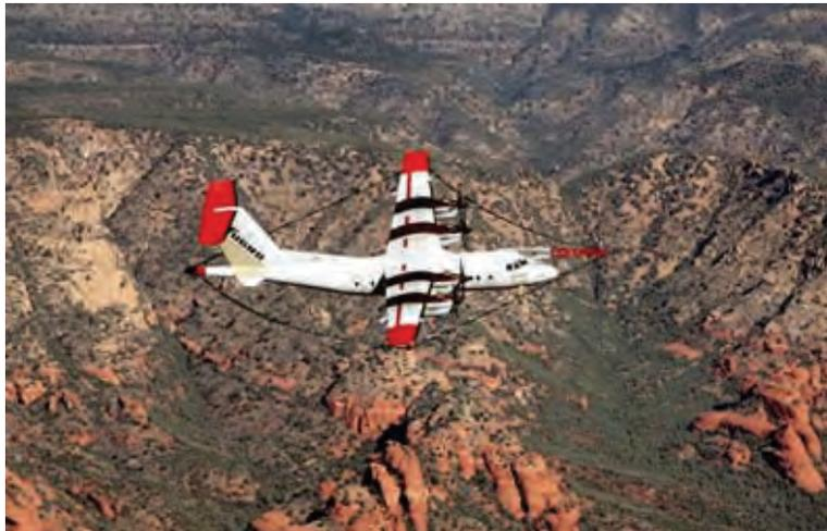
Figure 4-9: A fixed wing time domain airborne EM system. (Fugro Airborne Surveys)
