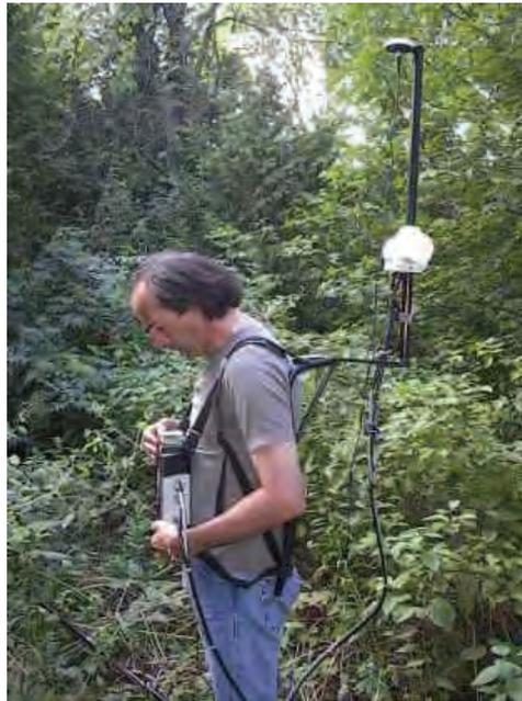
**Figure 5-4: GSM-19 Overhauser “Walking Mag” (TerraPlus Inc.)**
