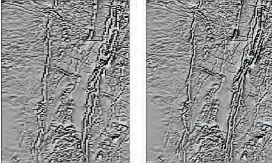
**Figure 4-7: Airborne magnetic data - total field (left) and gradient (right). (Fugro Airborne Surveys)**
