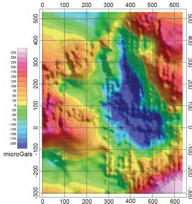
**Figure 5-3: A microgravity survey example in karst terrain. (Golder Associates Ltd.)**
