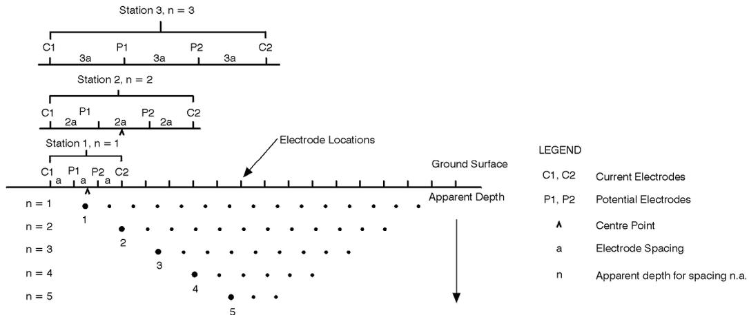
Figure 6-3: ERI measurements in a Wenner configuration using a multi-electrode array. (Golder Associates Ltd.)
