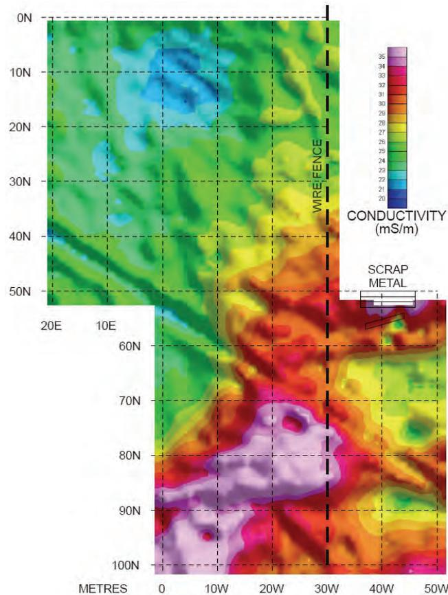
**Figure 6-7: Shallow EM survey to locate buried waste. (Golder Associates Ltd.)**
