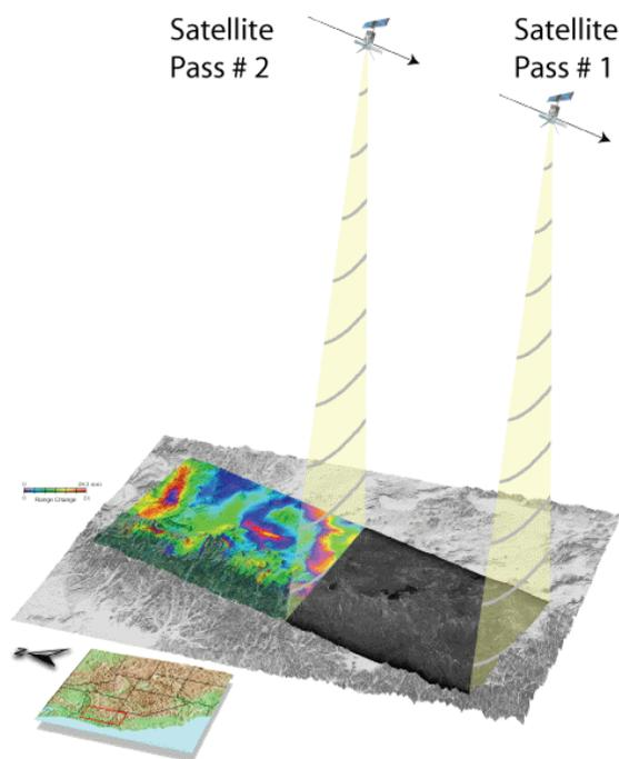
**Figure 3-3: InSAR image acquisition and resulting interferogram. (USGS)**
