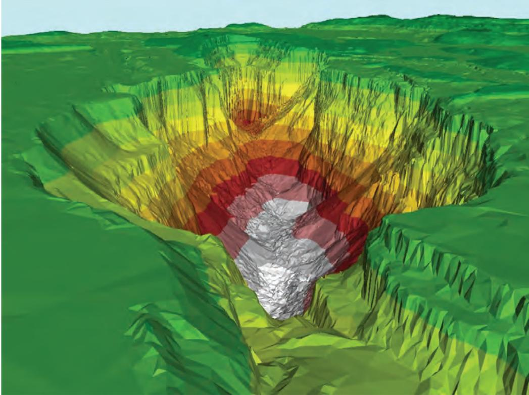
**Figure 4-3: An example of a DEM generated from airborne LiDAR data. (Terrapoint Canada Inc.)**
