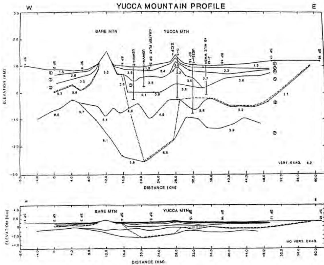
Figure 7-9: Crustal velocity model along the Yucca Mountain seismic refraction profile (Mooney and Schapper, 1995).
