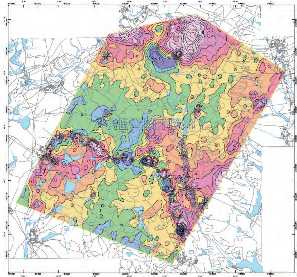
**Figure 7-18: Example total magnetic field survey results, Czech Republic. (McPhar Geosurveys Ltd., 2004)**
