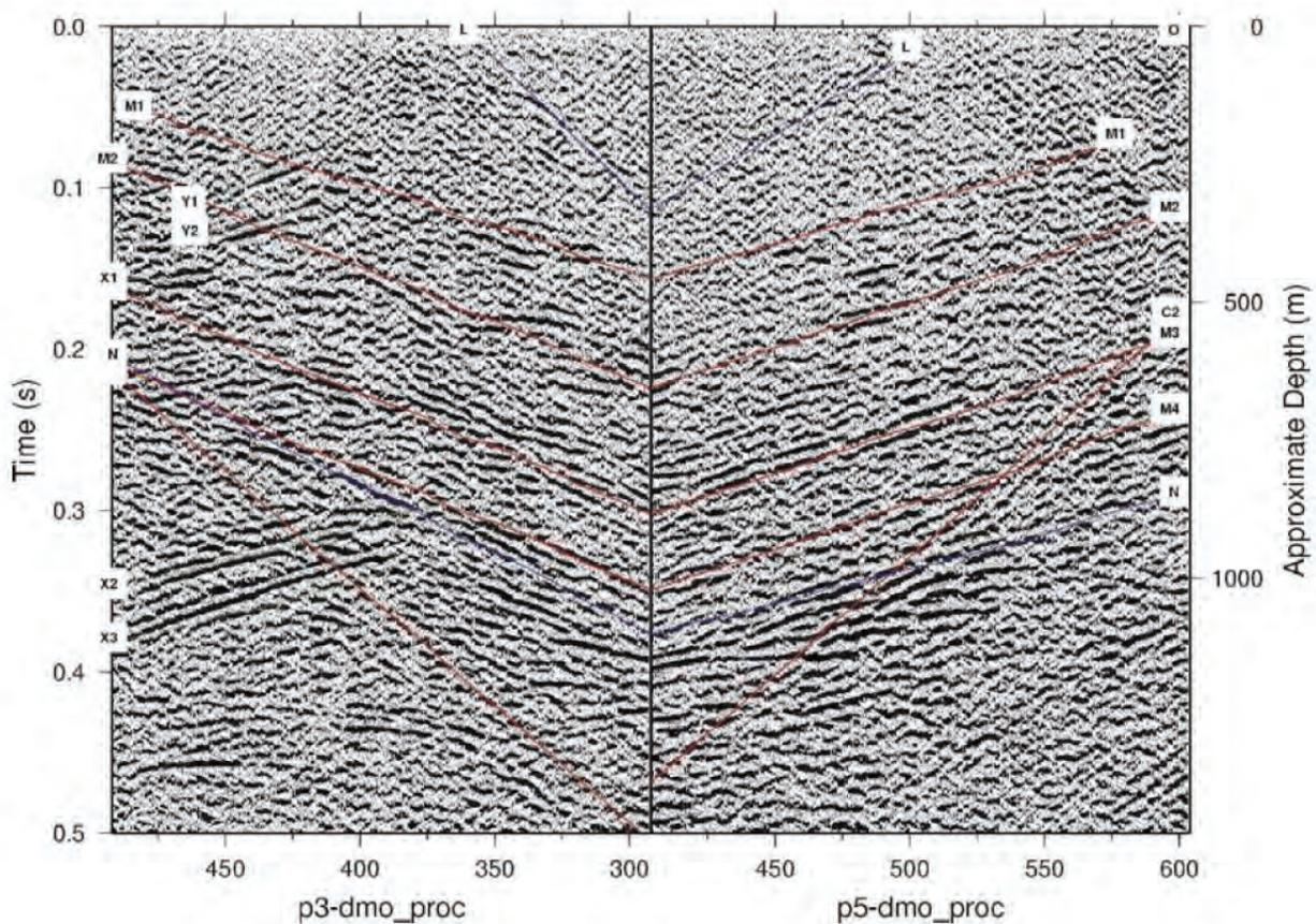
**Figure 7-3: 2D seismic reflection results at Laxemar in 2004 showing the correlation between profiles 3 and 5. (Juhlin et al., 2004)**
