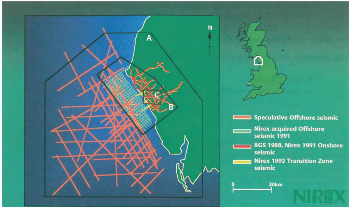
Figure 7-4: Investigation area at Sellafield showing the location of most seismic surveys. (Chaplow, 1994)
