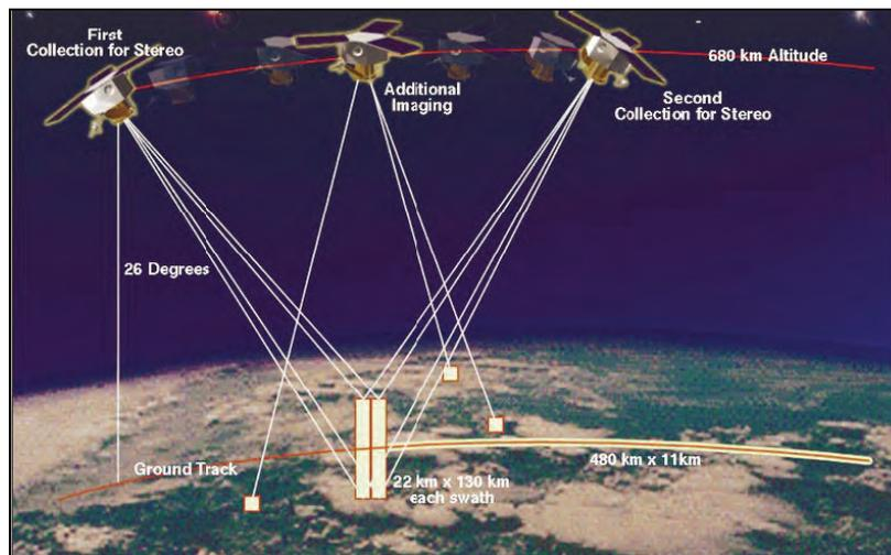
**Figure 3-2: Satellite imagery acquisition. (GeoEye Inc.)**
