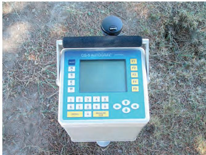
**Figure 5-2: The Scintrex CG-5 “Autograv” Gravimeter. (Scintrex Ltd.)**
