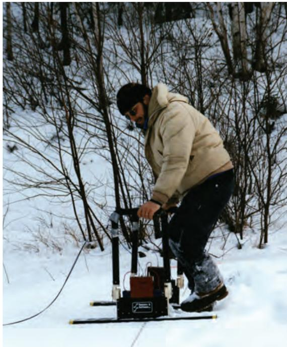
**Figure 6-5: Acquisition of 100 MHz GPR data (Golder Associates Ltd.)**
