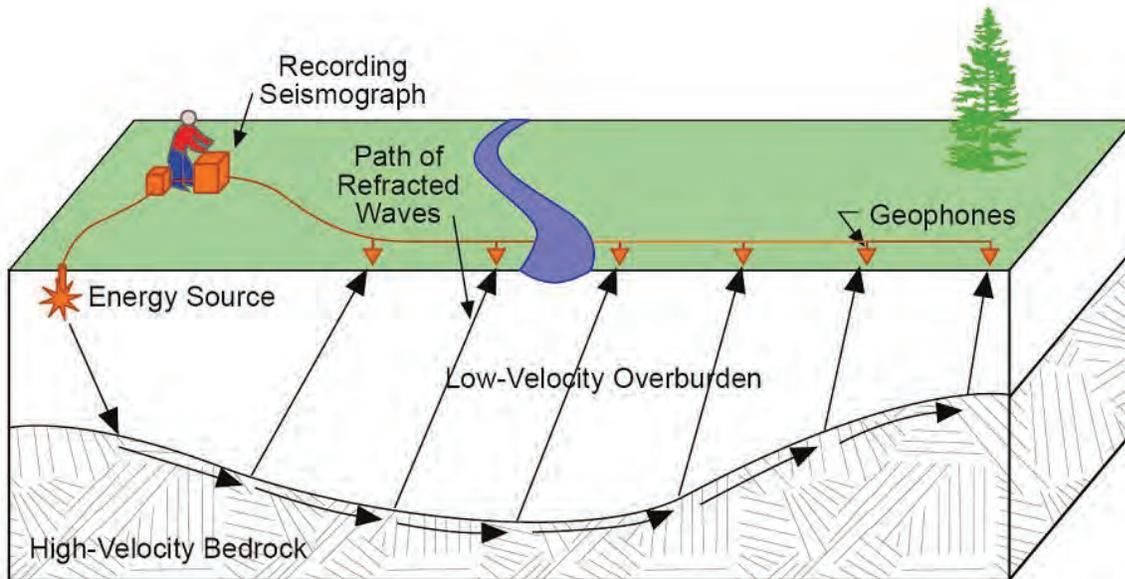
**Figure 6-1: Conceptual sketch of the seismic refraction method, showing the field layout and the path of a refracted wavefront (Golder Associates Ltd.)**
