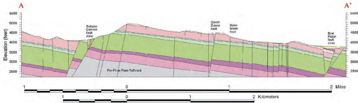
**Figure 7-7: Cross section showing the distribution of volcanic rocks at Yucca Mountain (DOE, 2002 modified from Day, Dickerson et al. 1998)**
