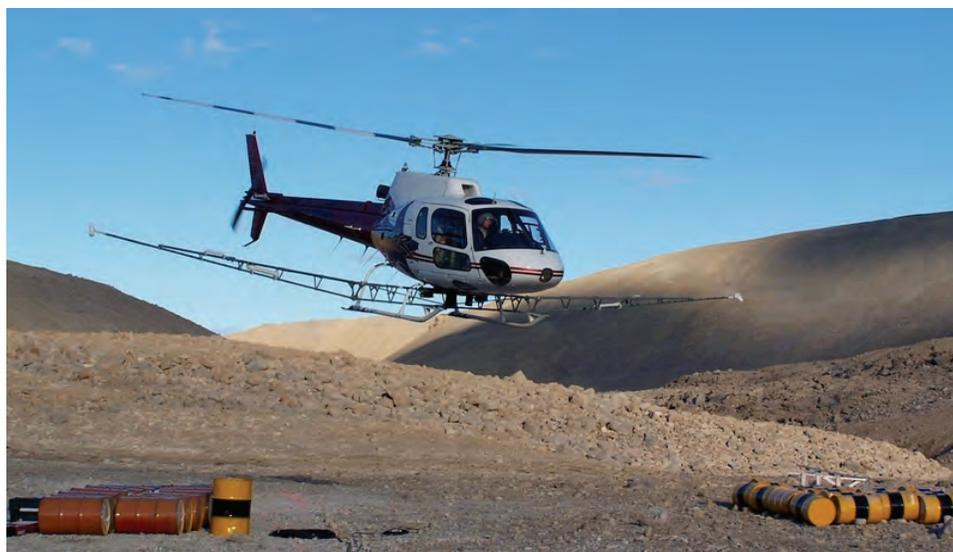
**Figure 4-6: A helicopter mounted horizontal gradient magnetic survey. (Fugro Airborne Surveys)**
