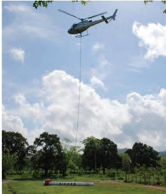
**Figure 4-10: A helicopter borne frequency domain EM system. (Fugro Airborne Surveys)**
