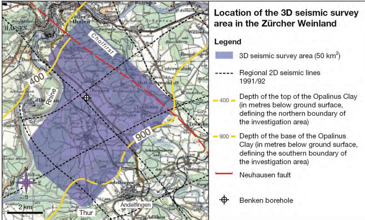
**Figure 7-12: Location of the 2D and 3D seismic surveys at the Zürcher Weinland site. (NAGRA, 2000)**
