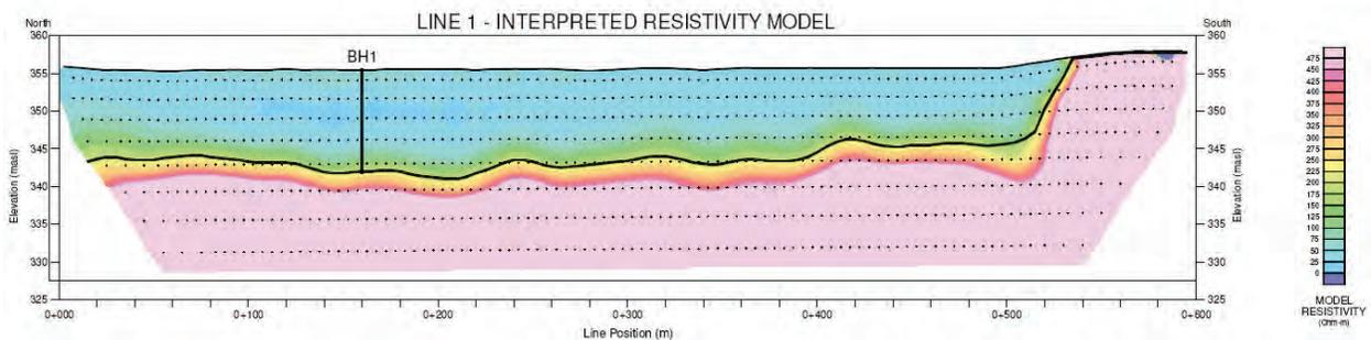
**Figure 6-4: Example ERI model section showing the inferred upper bedrock surface overlain by silt and clay soils. (Golder Associates Ltd.)**
