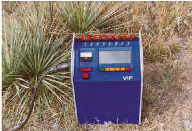
**Figure 6-9: VIP 3000 IP/Resistivity Transmitter (TerraPlus Inc.)**
